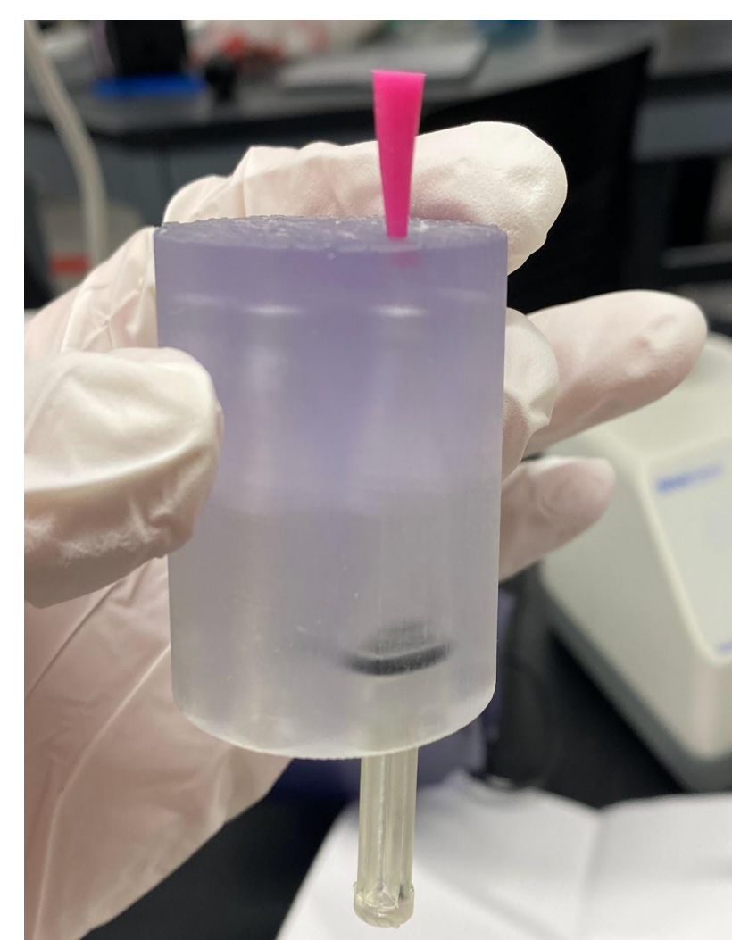
Figure 4.3: Final design loaded with fluorinert. No leaking is observed.
