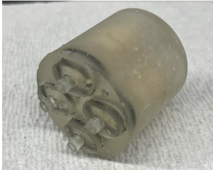
Figure 43. Loaded rat capsule for leak testing.
