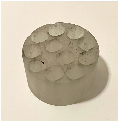
Figure 11. FormLabs Clear mice brain capsule for 11 mice brains with 9x7.5mm hole dimensions and 2.5mm diameter watermark hole.
