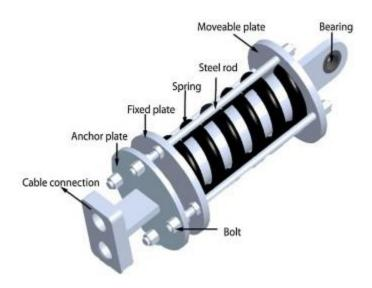
Figure 9: CAD model of the Spring Viscous Damper used in the damper-cable system [21].
