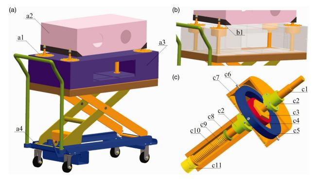
Figure 1: (a) an overview of the QZS vibration isolation system; (b) the installation view of the QZS isolators into the incubator control box; (c) the inside view of the QZS isolator [12].
