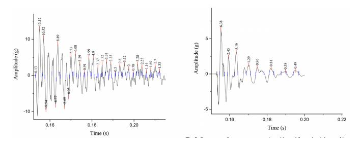
Figure 8: Damping curves for solid stainless steel (left) and the composite damper (right) [19]. Testing was conducted for this mechanism. Results can be seen in **Appendix B**.
