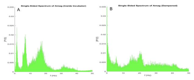
**Figure 1:** Power spectral density graphs for measurements (A) inside the incubator without the dampening prototype, and (B) inside the incubator with the dampening prototype.
