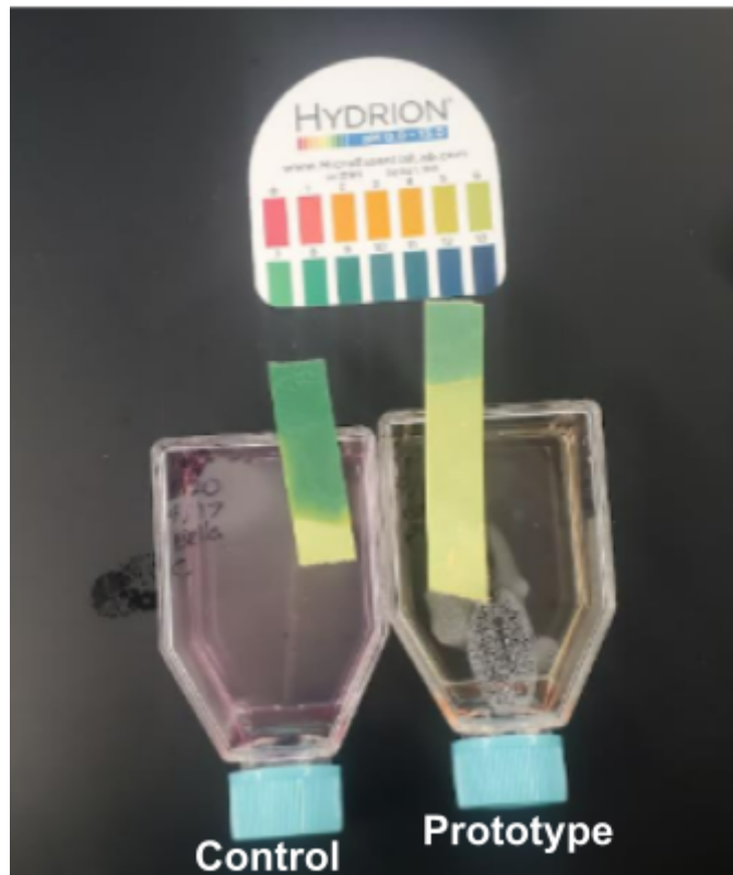
Figure 27: pH strips of control vs prototype at 3x the amount of CO 2 showing that the control had a pH of approximately 7 while the prototype had a pH of approximately 5. The yellow discoloration in the prototype flask indicates oversaturation of CO 2 .
