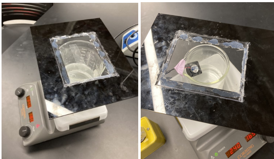
Figure 9: PDMS anti-condensation testing setup with and without a mini-fan
