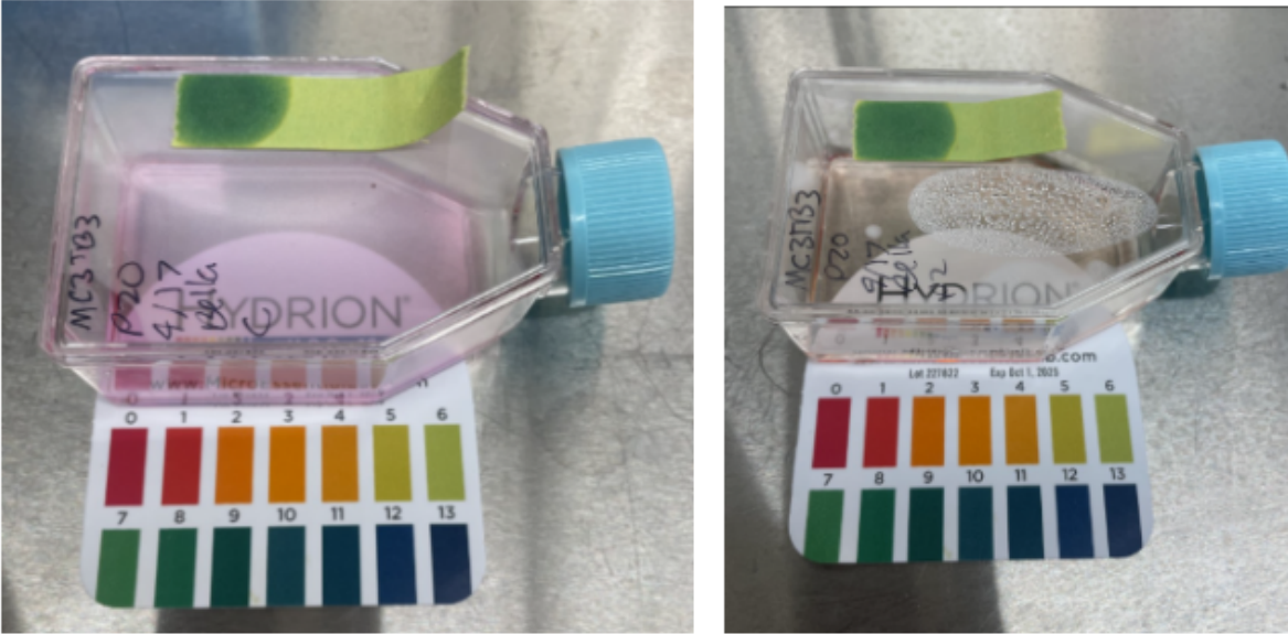
Figure 28: 2x the amount of CO 2 released. A: (Left) shows the control group in which the pH is approximately 7 and the color is a light pink. B: (Right) shows the prototype group in which the pH is approximately 6 and the color is orange.
