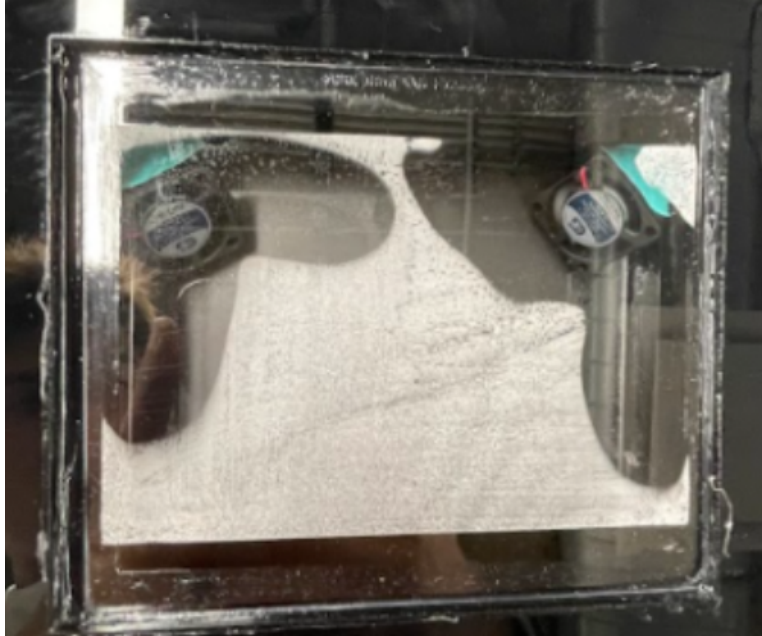
Figure 13: Image of the fog build up for the same side dual mini-fan placement after 45 minutes
