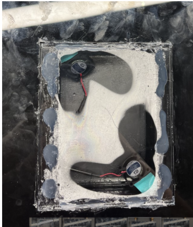
Figure 12: Image of the fog build up for the diagonal dual mini-fan placement 15 minutes after the lid was open and closed for 30 seconds.
