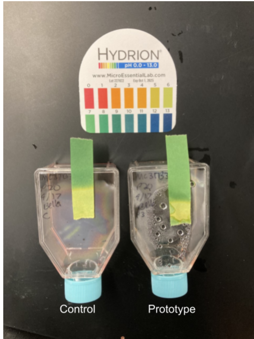
Figure 30: 1.75x CO 2 released comparing the control to the prototype. Both have around the same coloration and a pH of approximately 7.
