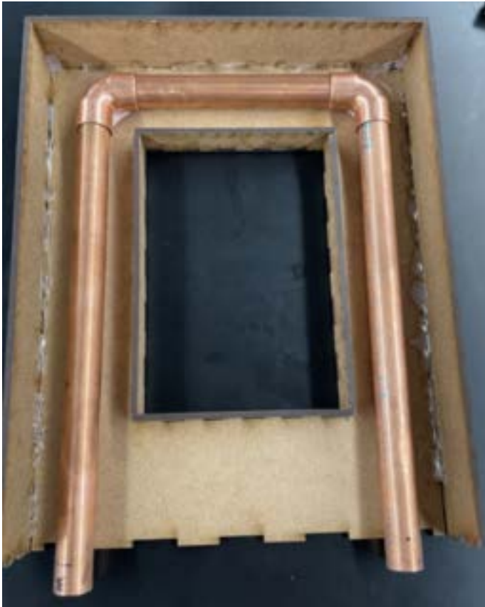
Figure 1: Inner copper tubing fabrication within the prototyped box.
