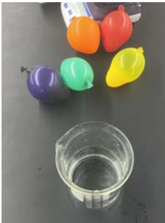
Figure 1: Photo of the filled balloons after the solenoid being opened for one second. Also shown is the beaker with water.
