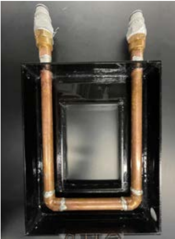
Figure 2: Top view of the new incubator box showing the caulking and copper piping.
