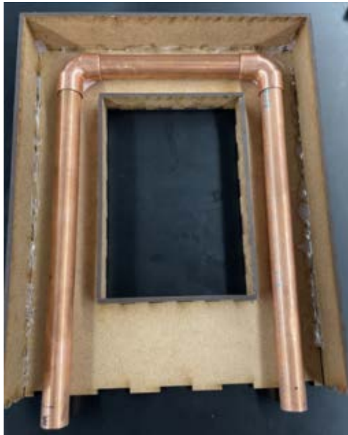
FIGURE 1: Cut copper pipe and L joints inside cardboard prototype to showcase fit (Yet to be soldered together)
