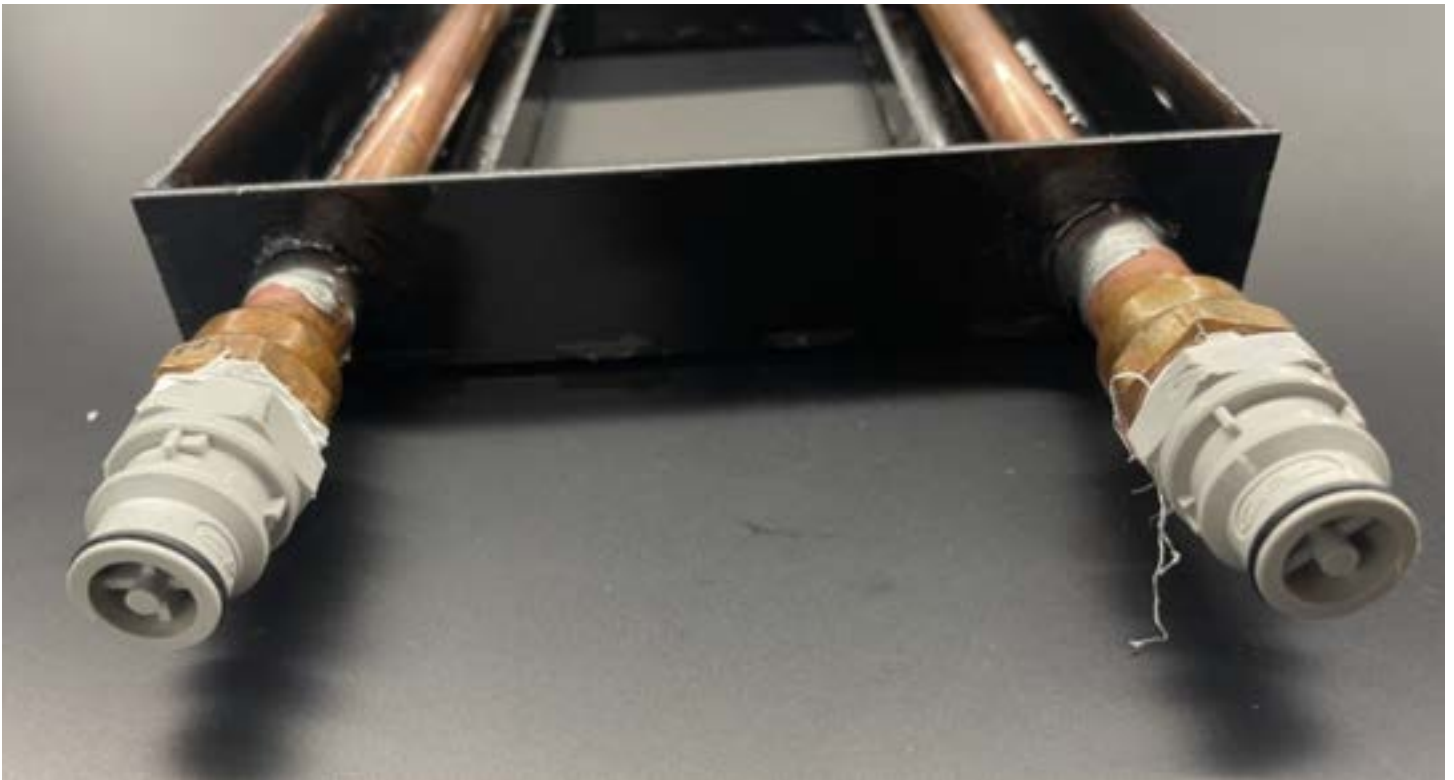
Figure 3: Side view of hose adaptors showing the new plumbers tape and caulk to prevent water leakage.
