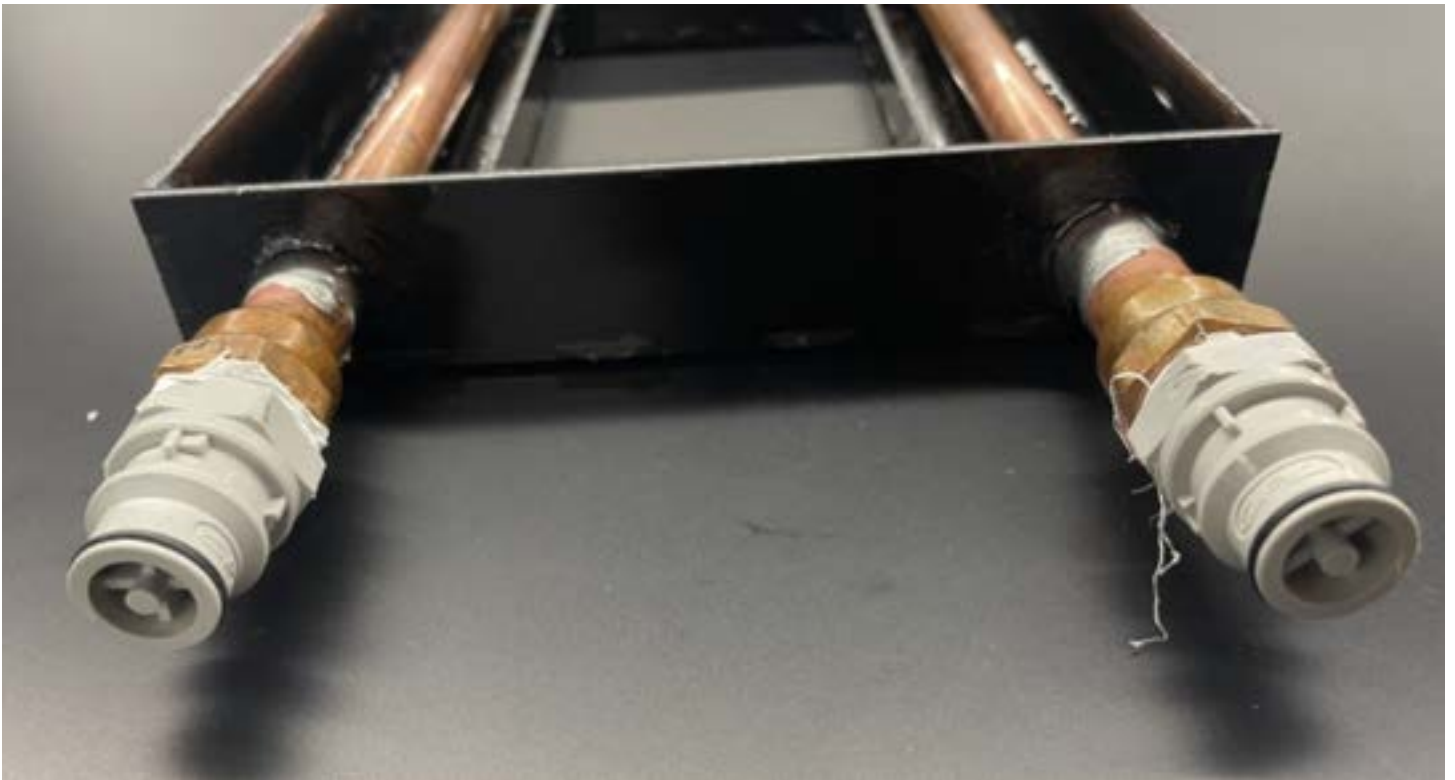
Figure 3: Side view of hose adapters showing the new plumbers tape and caulk to prevent water leakage.
