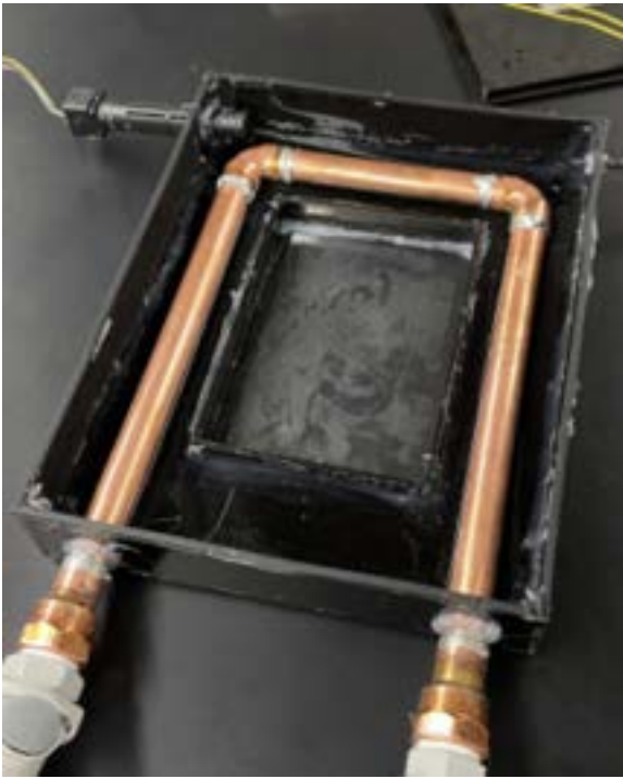
Figure 2: Photo of plumbing soldered copper tubing within the incubator box.
