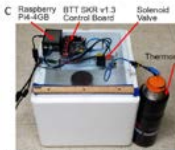
Fig 1. Schematic diagram and pictures of the components of device. (A) General schematic diagram of the device and setup. (B) Photo of the setup using a small plastic food storage container. (C) Larger incubator setup using a Styrofoam box that can be used with the same hardware. The latex balloons (orange) and a three-way connector covered with a flexible latex band (yellow) in the CO 2 line acted as passive venting features. This restricts a small positive pressure in the thermos to supply the CO 2 , but without the risk of excessive pressure build up inside the thermos.
