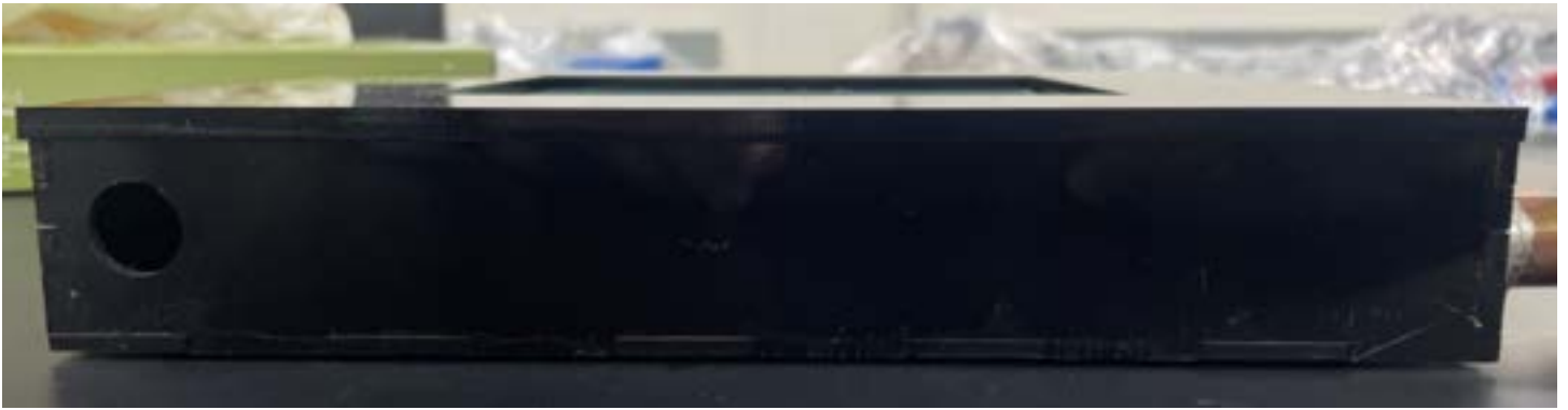
Figure 4: Side view of thick lid fabrication showing the size and tight fit on the incubator box.
