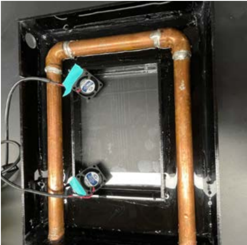
Figure 1: Inside of the box dual mini fan same side set up
