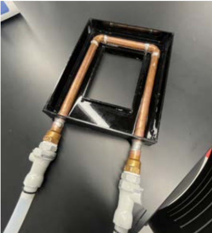
Figure 1: Aerial view of the newly fabricated incubator box connected to the heated water pump and contains a bed of water. No leakage.
