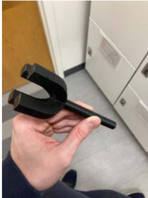
FIGURE 5: Final 3D Printed PLA Plastic Valve holder:
