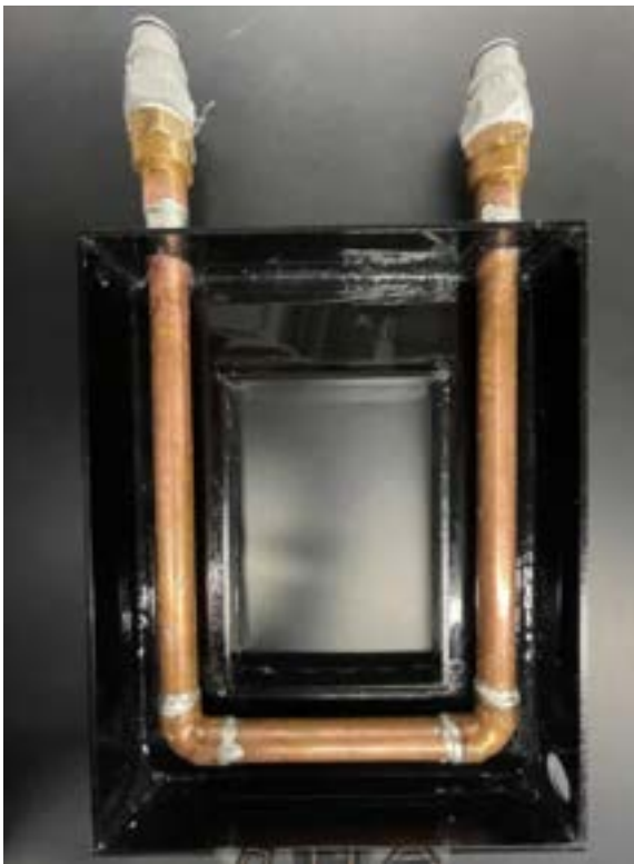
Figure 3: Newly fabricated box with waterproof silicone caulk seals.
