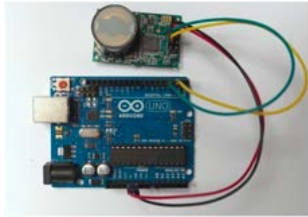
Figure (2): CO2 Sensor and Arduino Control
