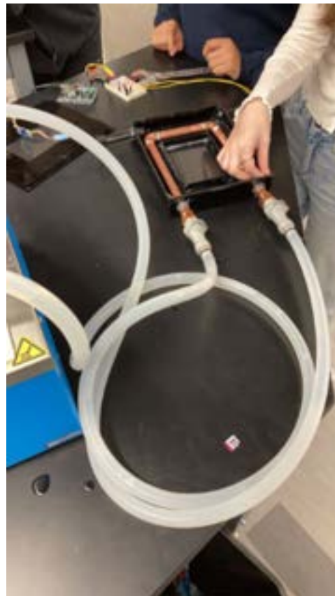
FIGURE 3: Leakage testing Setup
