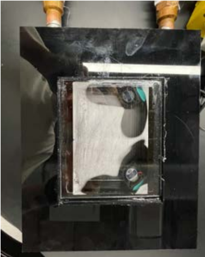
Figure 5: 15 minutes after lid opening and closing of same side dual mini fan set up testing
