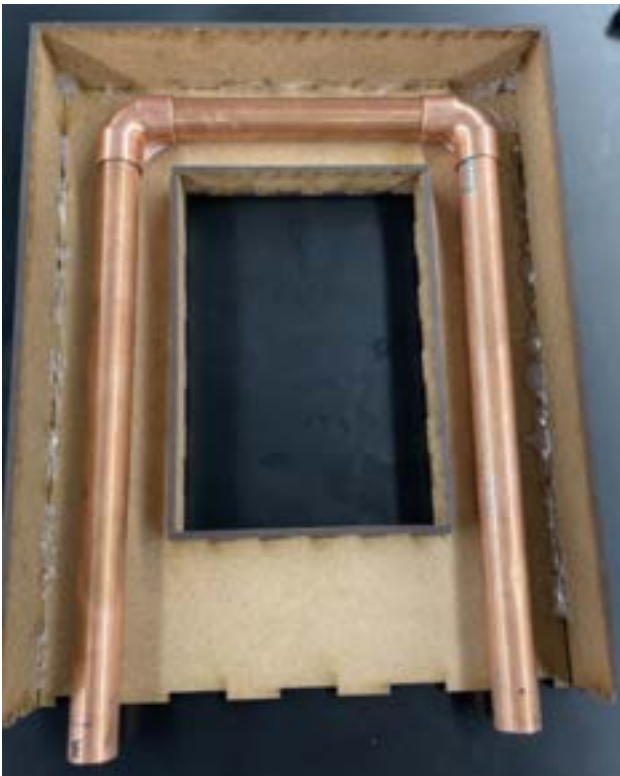
Figure 2: Inner copper tubing fabrication within the prototyped box.
