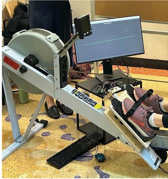
Figure 23. Rower's feet strapped into footplate with GUI on monitor.
