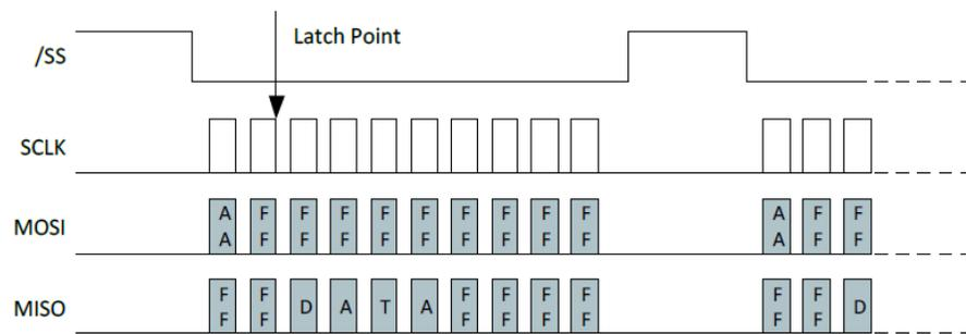
Figure 17. Timing diagram of the SPI communication to and from the p3 angular encoder. [23]
