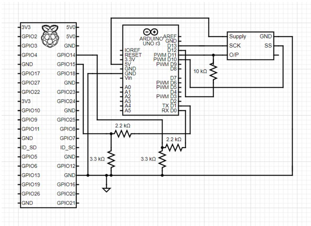
Figure 19. Circuit diagram of the final design with the Raspberry Pi (left), Arduino UNO (middle), and p3 angular encoder (right).
