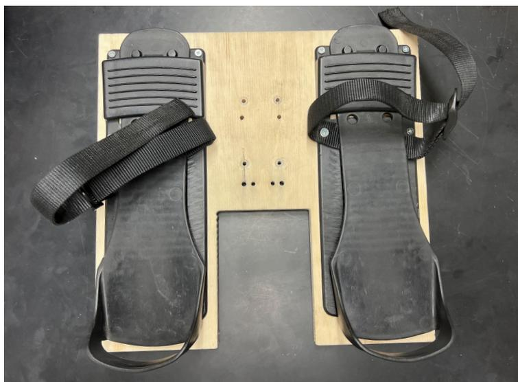
Figure 25. Top plate with Flexfeet attached.
