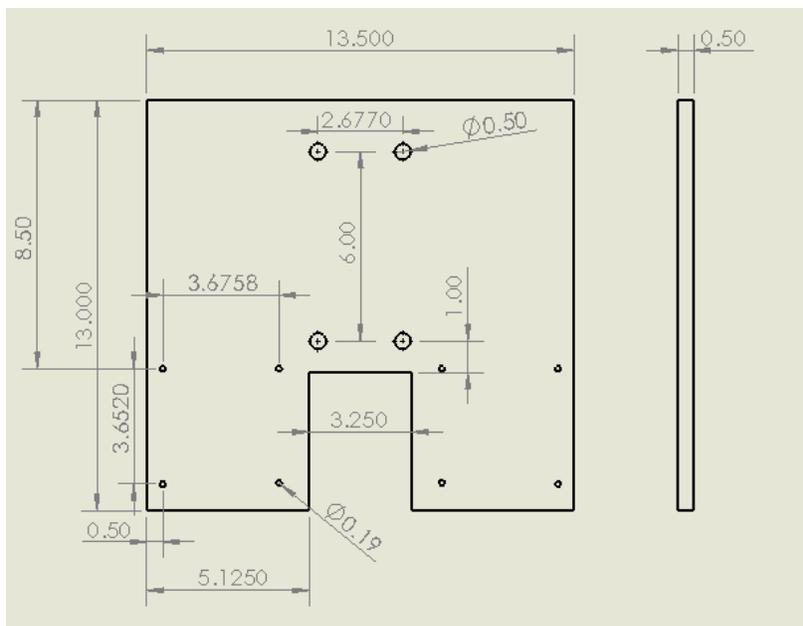
Figure 15. Dimensions of base plate in inches.
