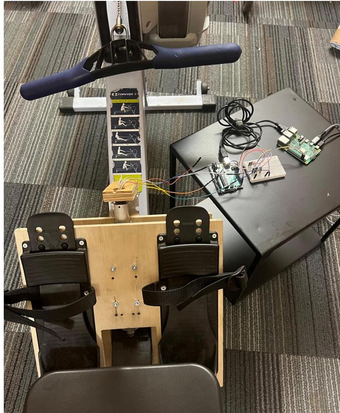
Figure 22. Footplate mounted on ergometer with accompanying circuitry.
