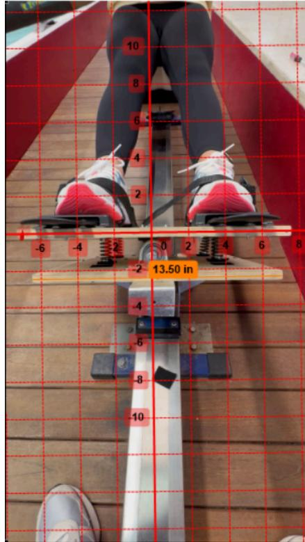
Figure 35. Side view of the footplate during testing imported in Kinovea with coordinate system.
