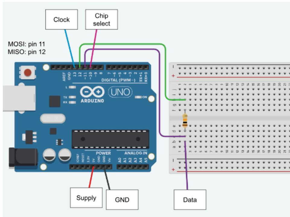
Figure 18. Fritzing diagram showing the connection of the P3 encoder wires to the Arduino Uno SPI pins with a 10 kOhm resistor.
