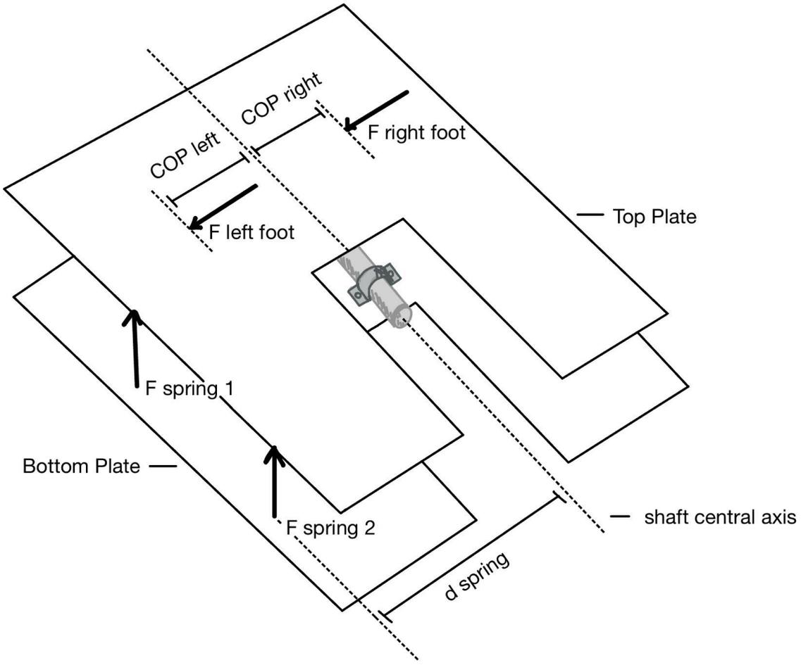
Figure 12. Free body diagram of footplates.
