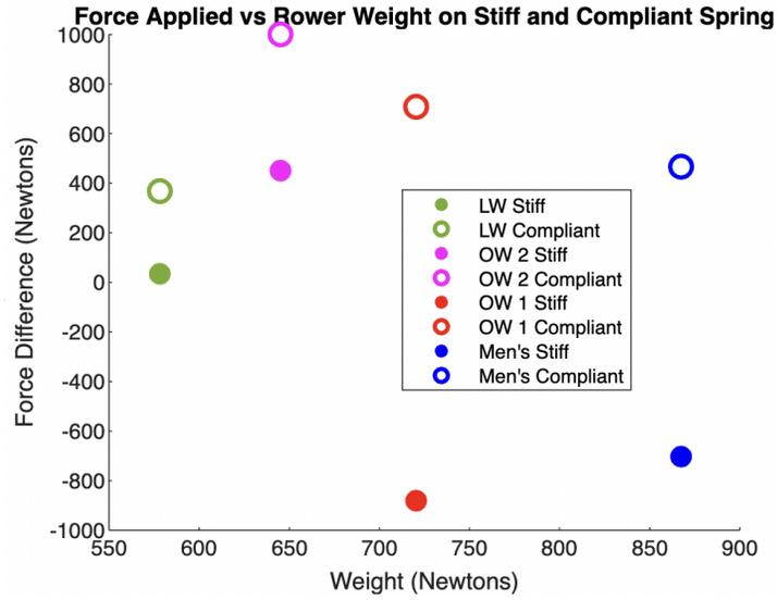
Figure 37. Force Difference vs Athlete Weight on Stiff and Compliant springs.
