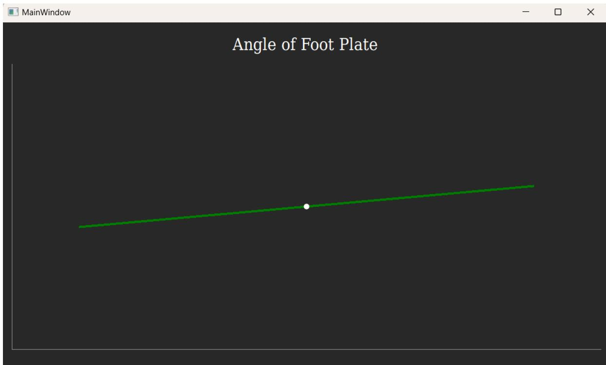
Figure 29. GUI showing the real-time angle of the top footplate using angle data from the P3 encoder.
