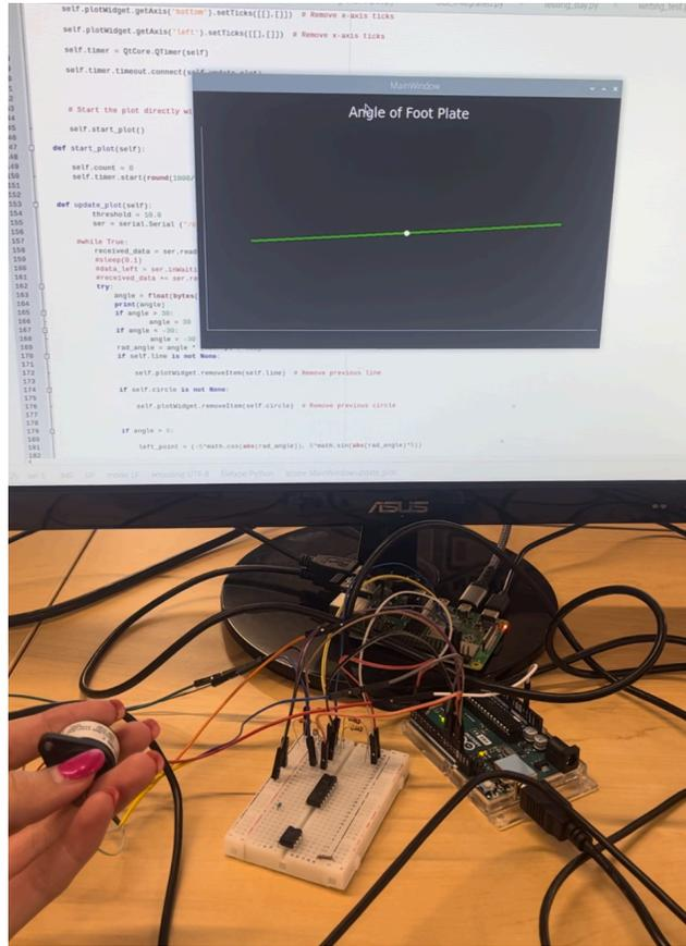
Figure 20. GUI showing the real-time angle of the p3 angular encoder shaft.
