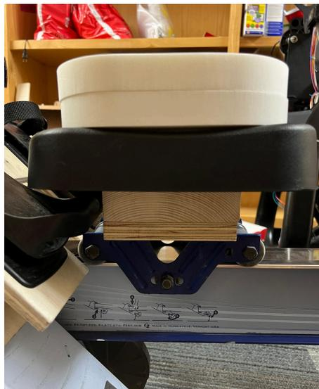
Figure 26. Adjusted seat height with wooden block and additional seat pads.
