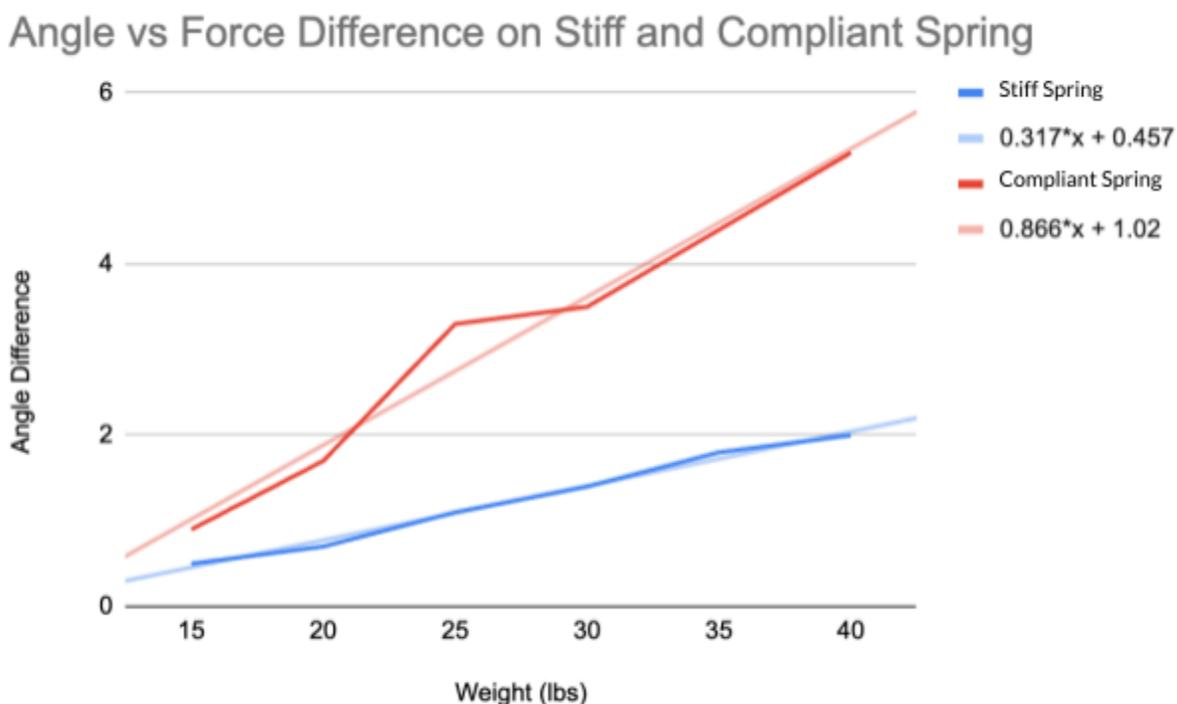
Figure 34. Angle vs force difference on stiff and compliant springs with the line of best equations.
