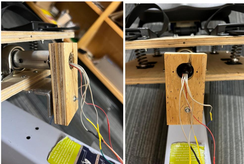
Figure 28. Side view (left) and front view (right) of angular encoder and mount.
