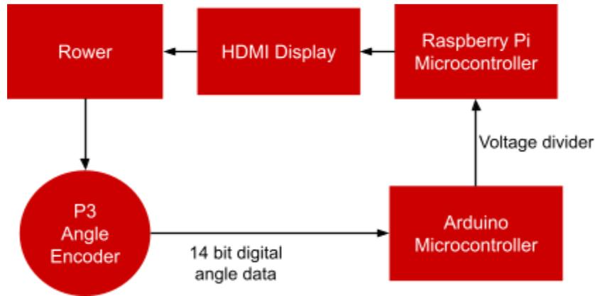
Figure 21. Logic diagram of the circuit providing real-time feedback to the rower.
