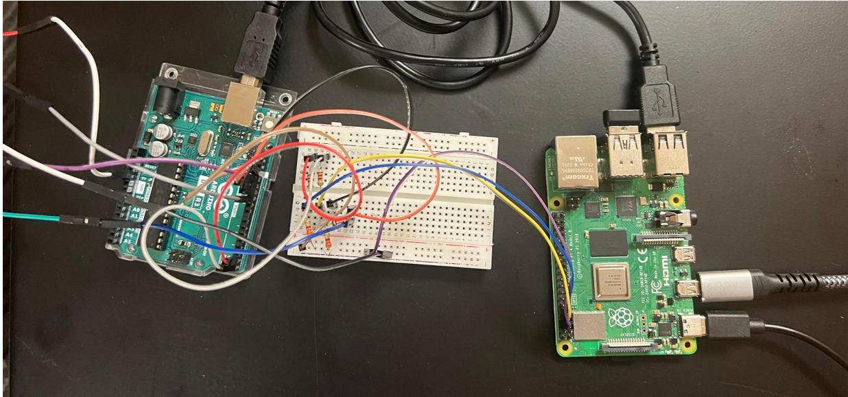
Figure 27. Arduino (left), breadboard with voltage dividers (center) and Raspberry Pi (right).
