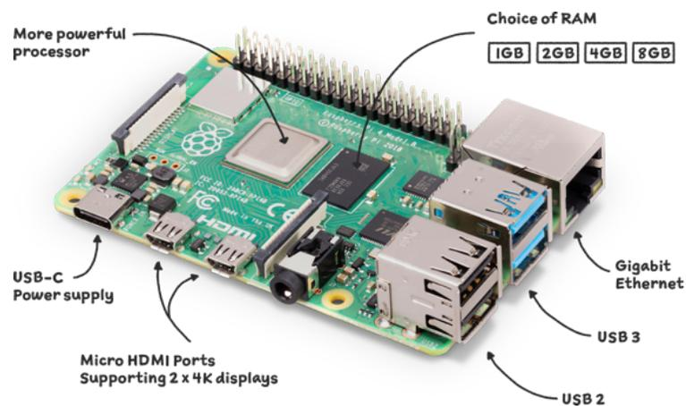
Figure 11. Raspberry Pi 4 Model B [19].
