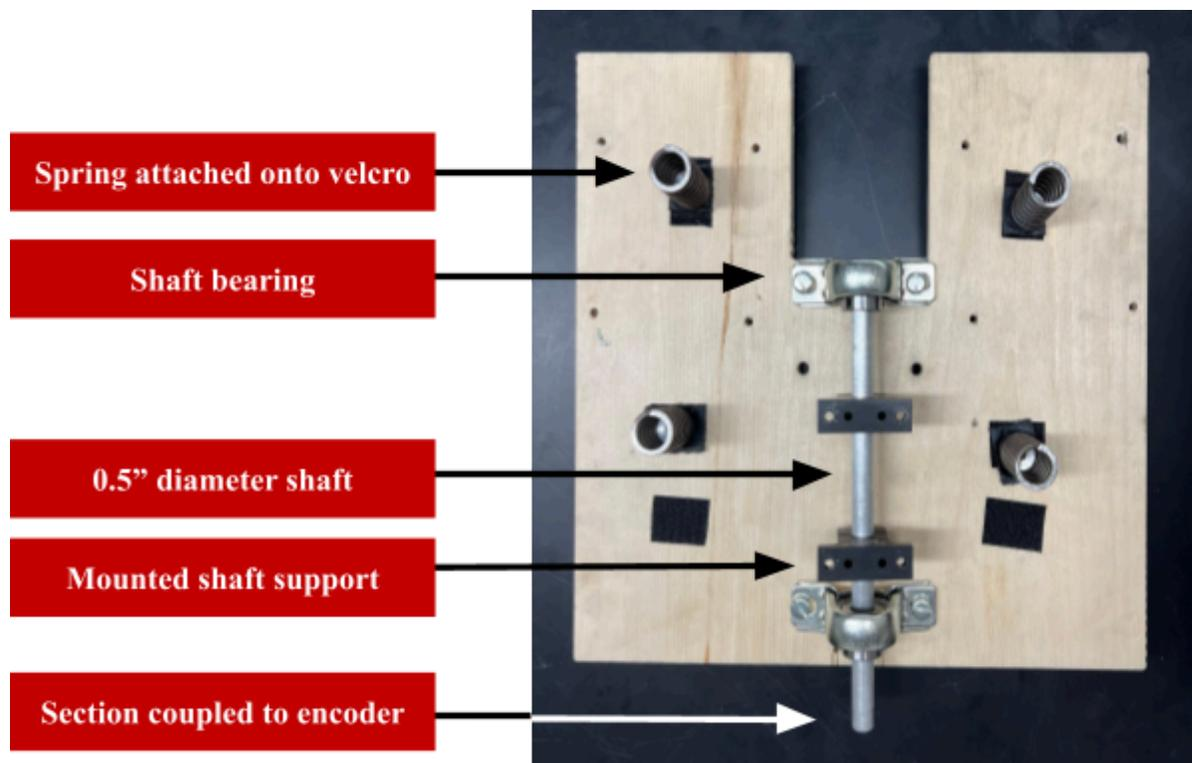
Figure 24. Bottom footplate with components.
