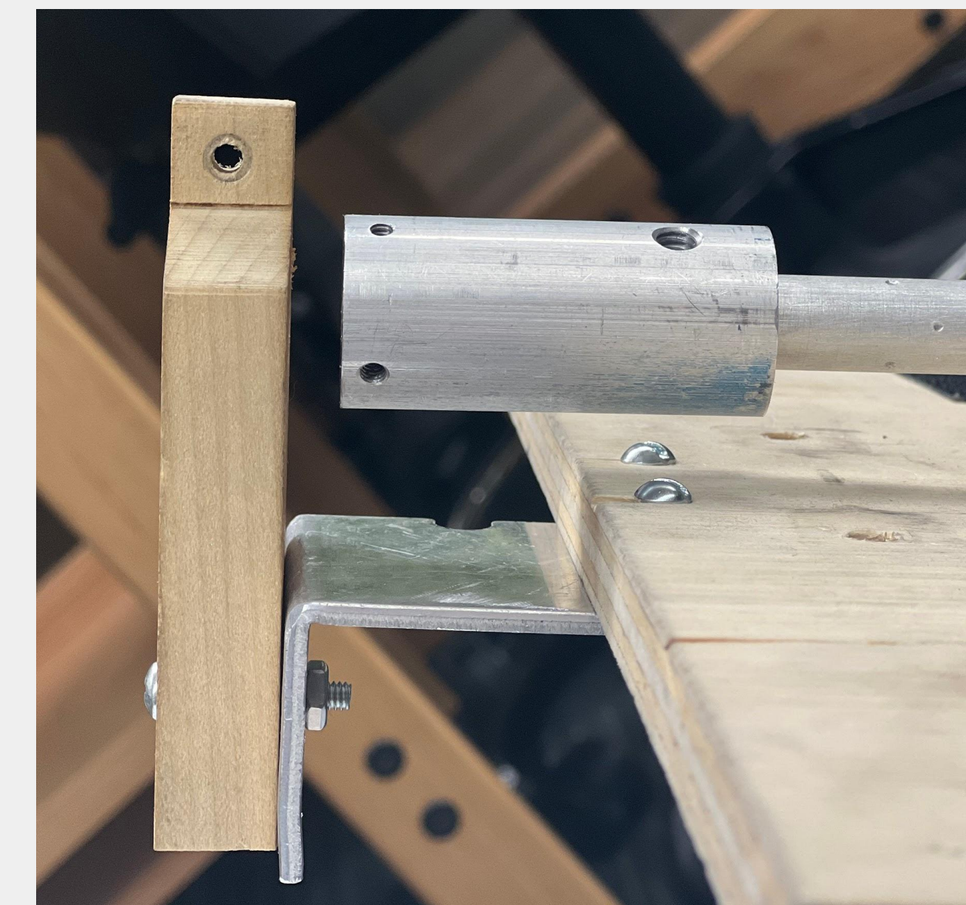
Figure 2. Angular encoder mount and coupling
