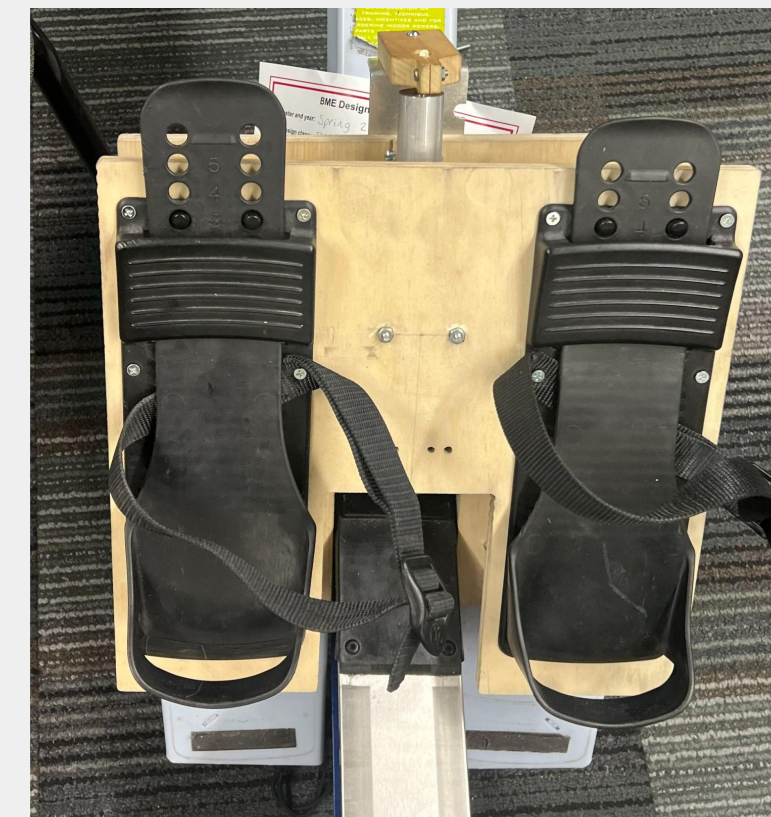
Figure 3. Front view of top plate bolted to flex foot and foot plate
