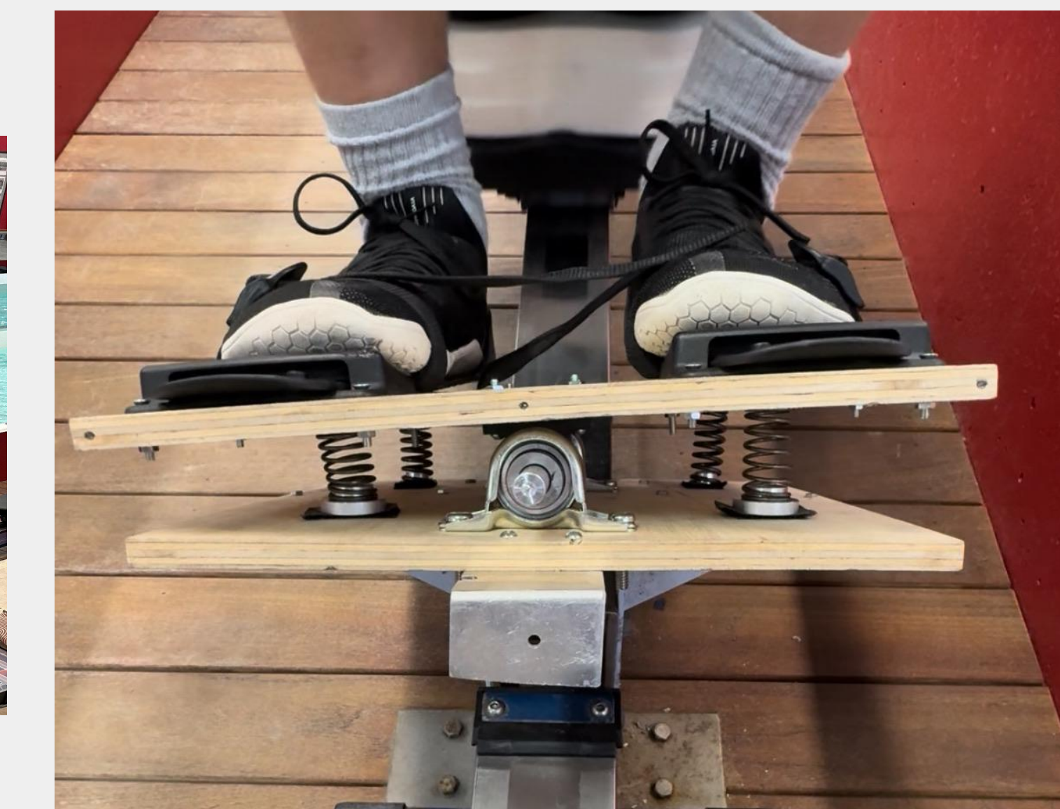
Figure 13. Men's rower on pivot design
