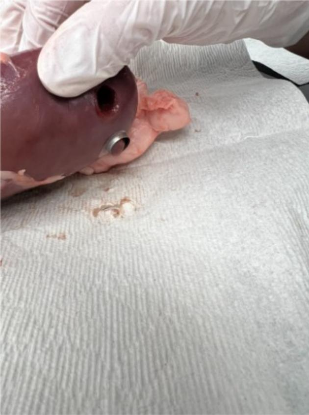
figure 4: device struggling to get through with fat attached
