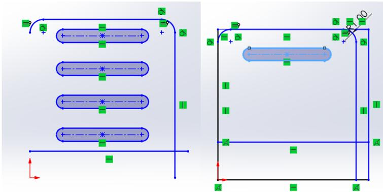
The bottom of the footplate. Left is just the cuts for the water jet, the right is some of the cuts with a model of the square plate.
