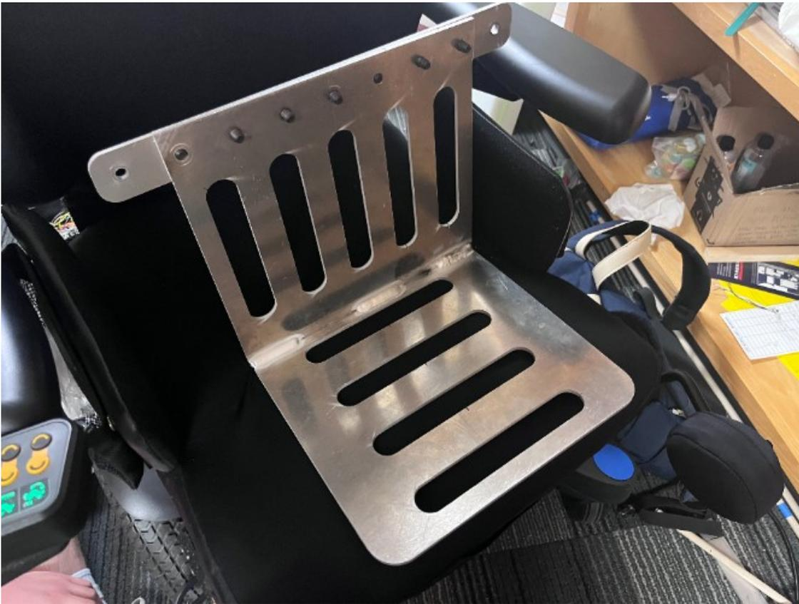
The waterjetted top and bottom aluminum plates are welded together, and an additional bar are screwed to the back of the top plate to be fitted on the wheelchair.
