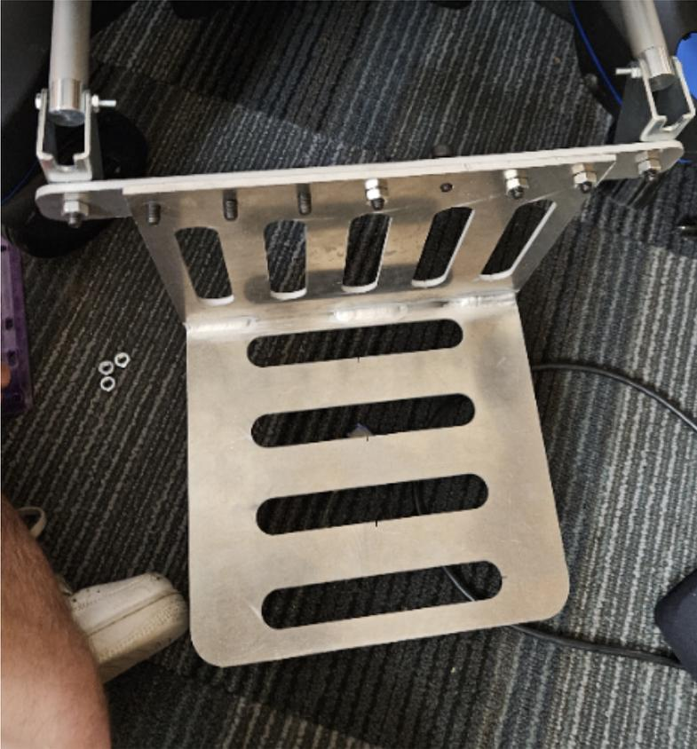
To remedy this issue the brackets were cut with a steel band saw to hug the actuator cap much closer to reduce the space and bending ability. Then carefully measured holes were drilled with a drop drill to but a screw through the actuator cap.
