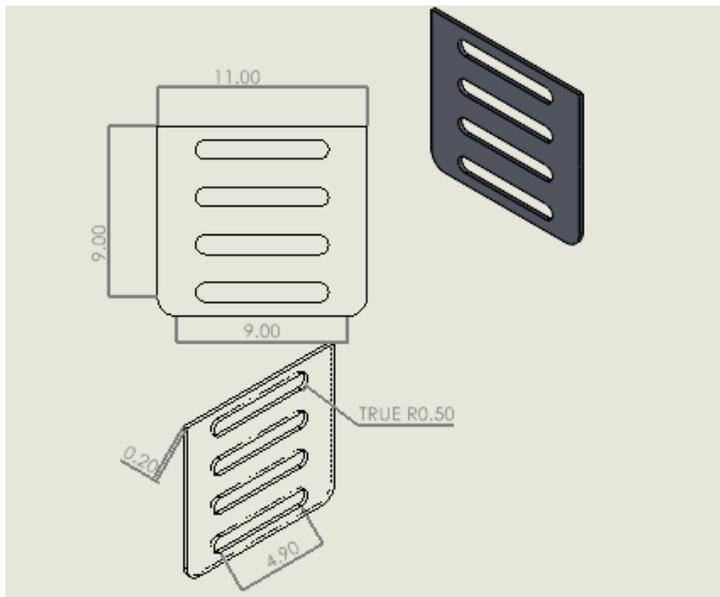
The figure above is the bottom of the footrest that the feet are placed on
