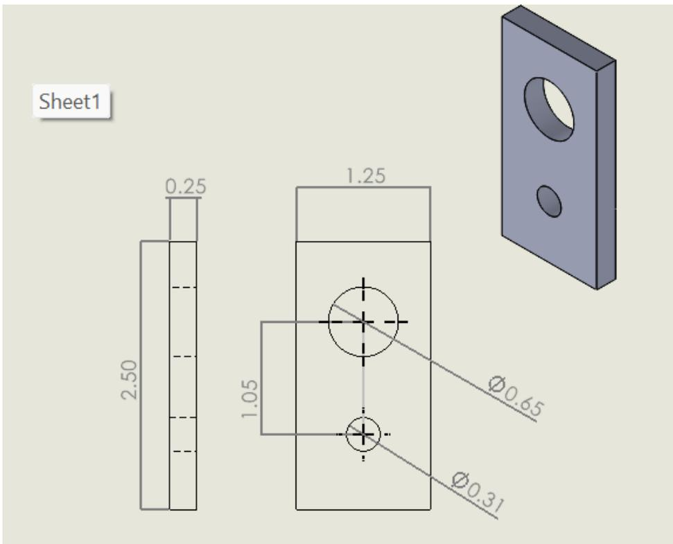
The bigger hole connects to the actuator and the smaller hole connects to the bar of the footrest and the lack of distance between the holes doesn't allow for much bending at the connection point.
