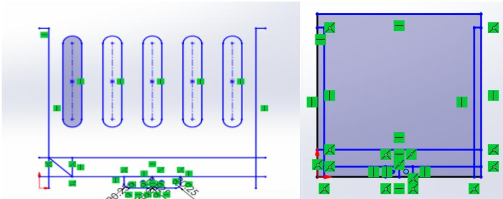
The top of the footrest. The left is the cuts of the water jet, the right has the model of the square plate, without the holes cut in.
