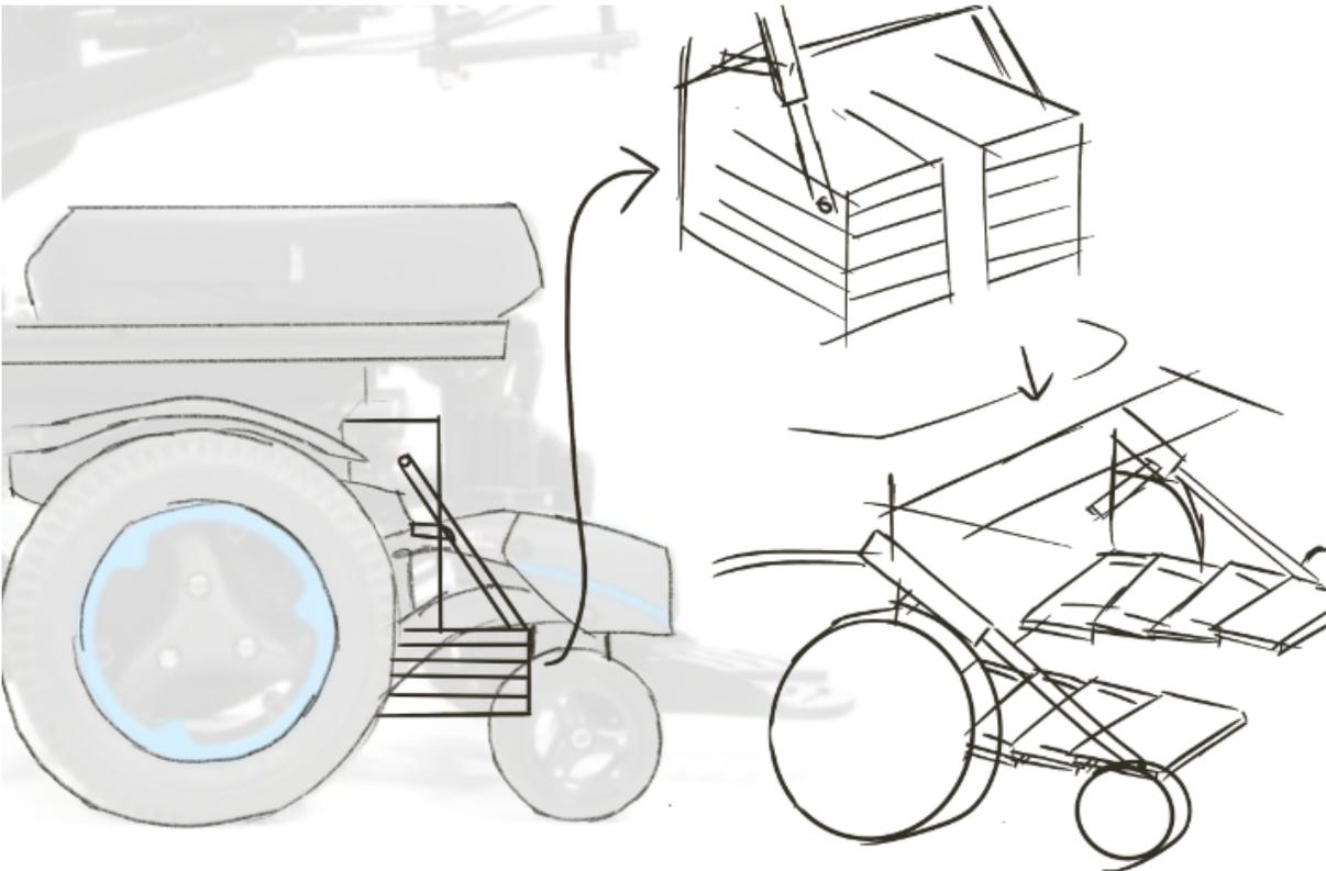
The layers of footrest slide on top of each other to extend. Retracts when not needed. All things will be placed underneath the chair and not interfere with the user.
