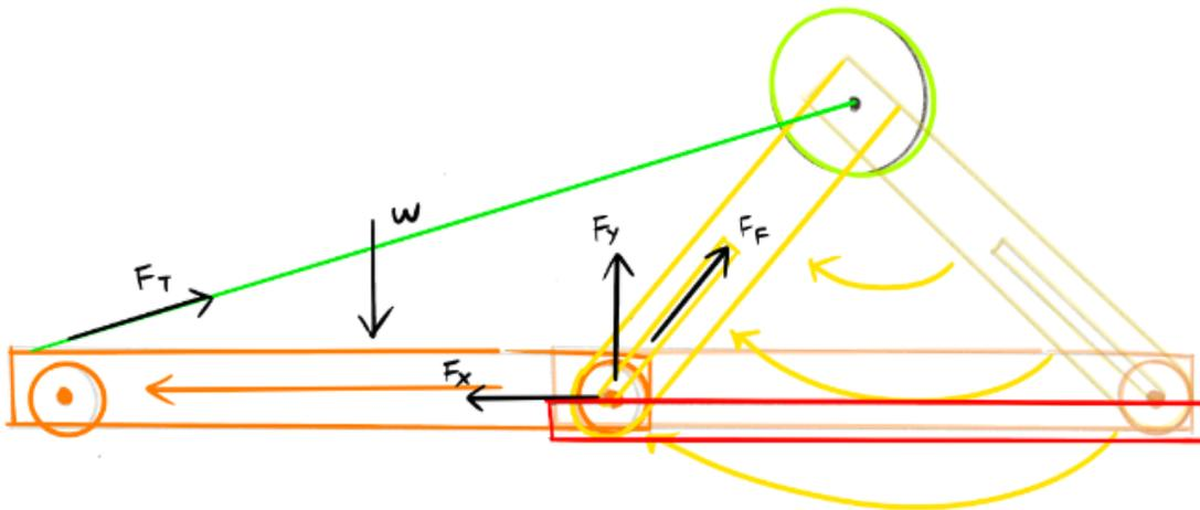
This design consist of a motor swing arm. The yellow piece is the swing arm with track cut out to allow connection to the footrest piece (orange). The footrest itself is connected with wheels, on the track on the side (red). The Green wire is providing tension to overcome the large moment produced by the weight. This is still a preliminary design and not perfectly though through.
