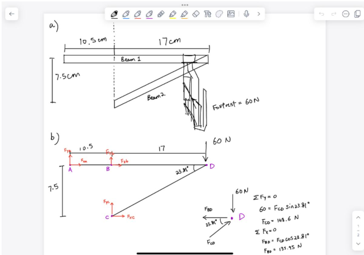
In this triangular support design, which uses two beams oriented in a triangle to support the footrest itself, and the leg+foot weight from the patient. It is determined that there will be two similar design, one on each side of the wheelchair for symmetrical purposes. One design must held 60 newtons of force at the end point. Using static equilibrium analysis, it is found that beam 1 is in 136N of tension, and beam 2 in 150N of compression. Shear stress in both is unknown and need to be solved.
