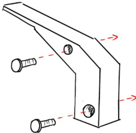
First image is the back holder, which uses screws already on the wheelchair for attachments. The holder lines up with these holes and connects to the linear actuator.
