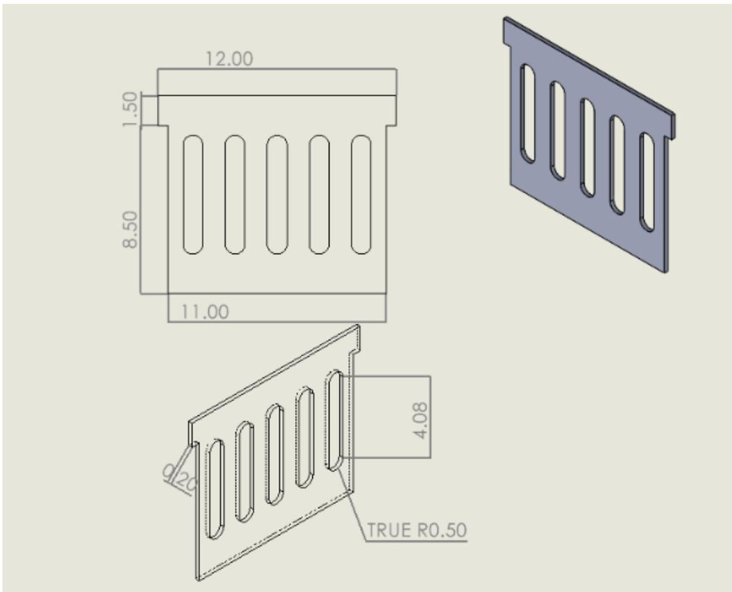
Figure above is the back that connects to the footrest, originally designed to be welded to small tabs that had holes in them like below
