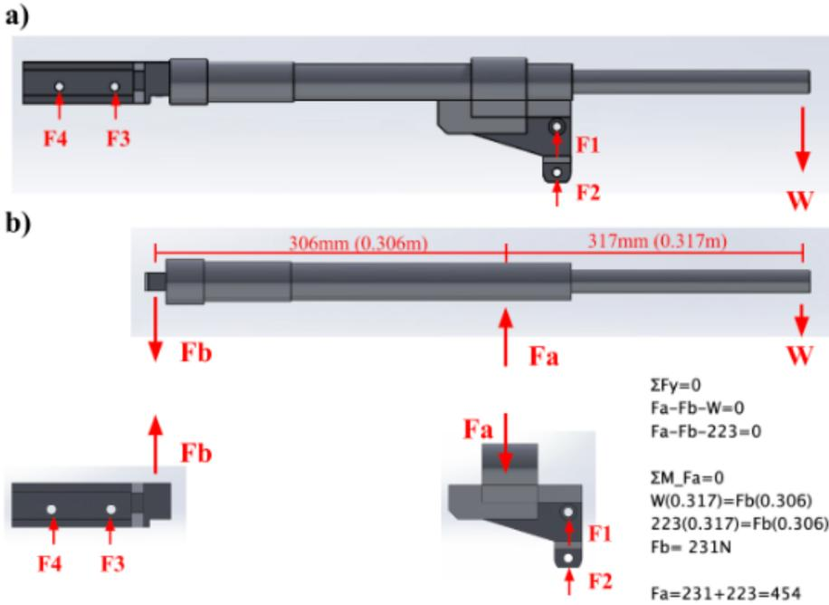
FigureX- force distribution of the linear actuator and holder support system (both actuators). a) single body force distribution b) force distribution by parts. Note: this is only a visual representation of the scenario and thus the extension of the linear actuator is not exactly to scale and the only supports are the front and back holder.  $W=223\text{N}$  (maximum applied force from bending test to both linear actuators).  $F_a=454\text{N}$  and  $F_b=231\text{N}$ .  $F1-4$  are arbitrary.
