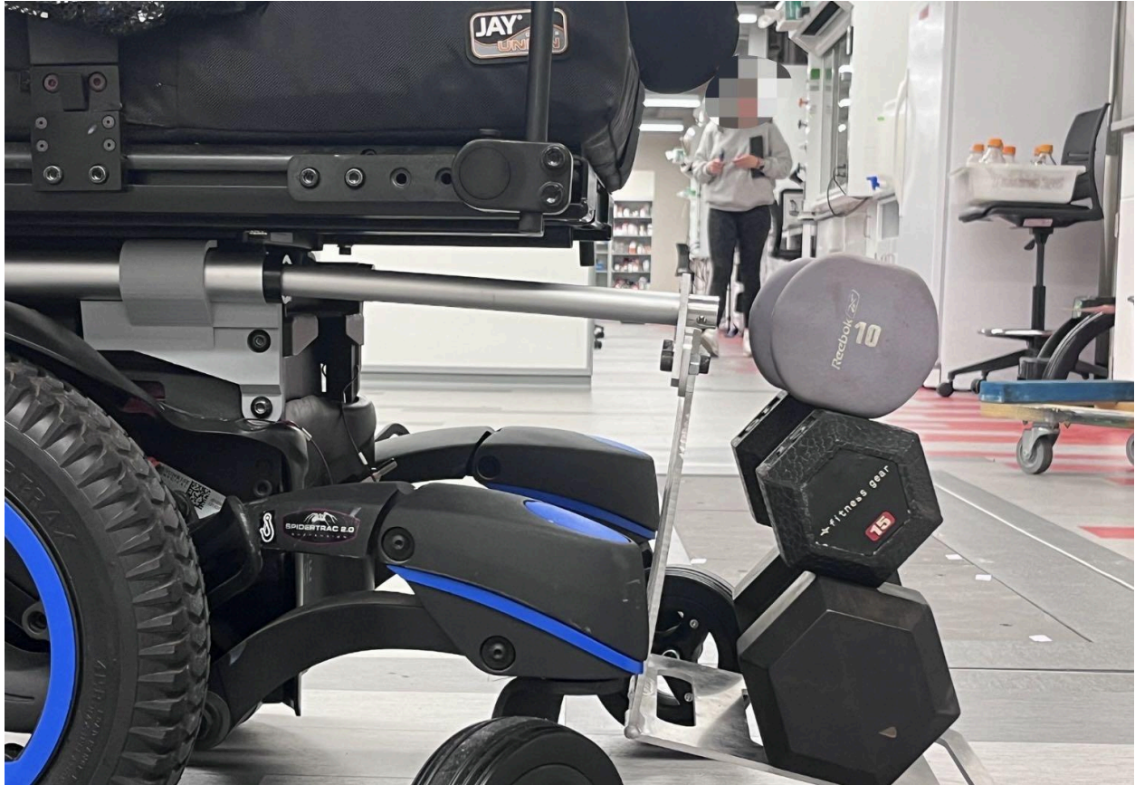
Figure 10.: Linear actuators are extended to around 250mm and various combinations of weights are put on the footrest and allow the linear actuator to bend
