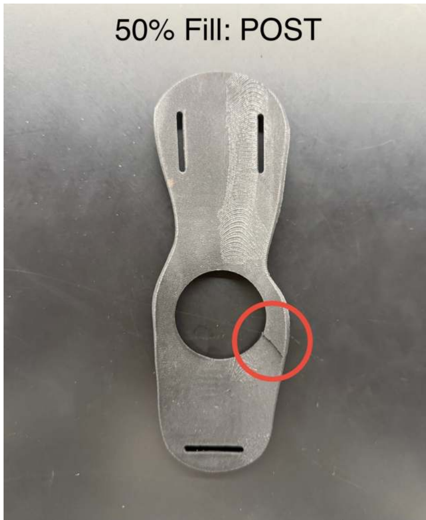
Every specimen failed in this area
