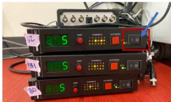
Figure 1. A.) Amplifier boxes for the in-ground force plates. The blue arrow indicates where the power switch is. B.) Bertec Acquire 4 software for data collection of force plate data.
