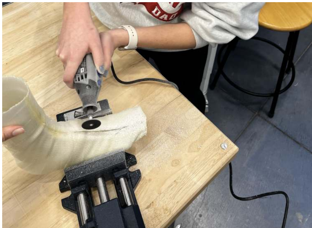
cutting the cast with a dremal, secured by a vise.
