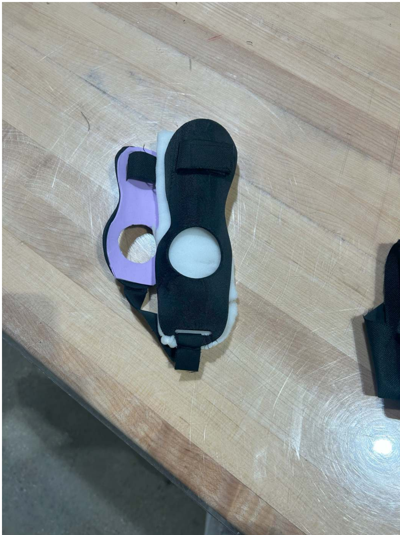
Close-up of the brace. To attach the white foam we had sewing into the foam and into the holes of the rigid support. It is very sloppy and we will regroup with the team to brainstorm better attachment ideas
