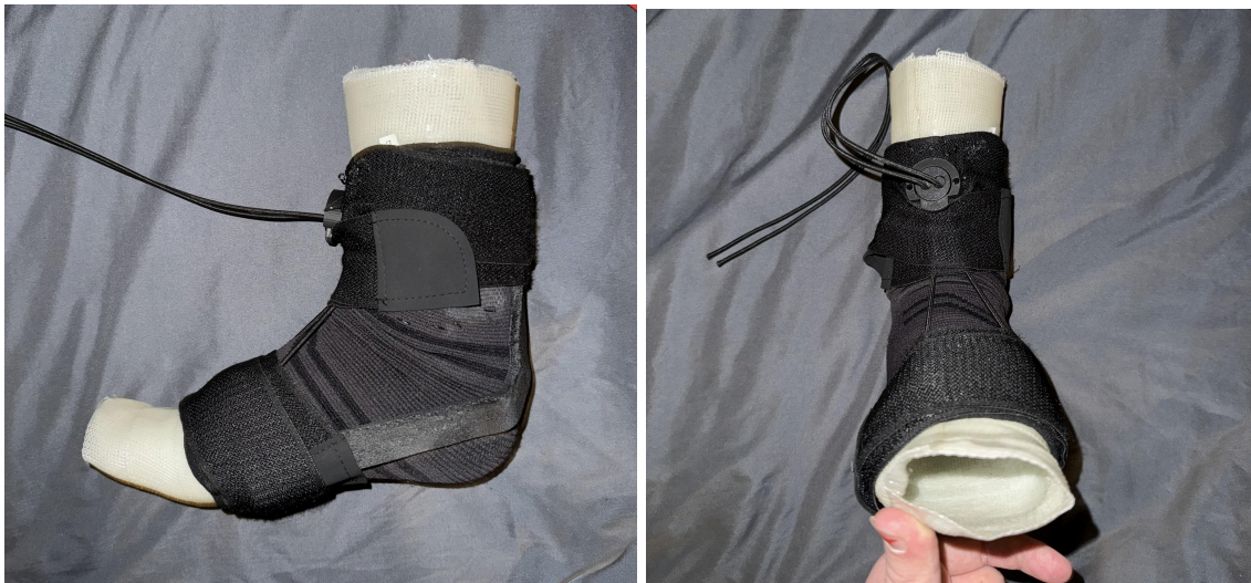
Figure 14: Bungee Brace Assembly, Lateral and Anterior Views.
