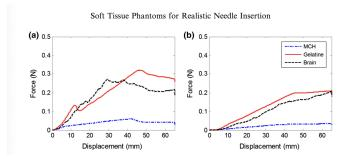
Figure 2: Mean forces of the needle for insertions and reinsertions into MCH, gelatin, and porcine brain.
