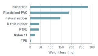
Figure 1: Abrasion resistance of materials is measured by the weight loss of a specimen in a standardized wear test. This figure depicts different materials and their abrasion resistance.
