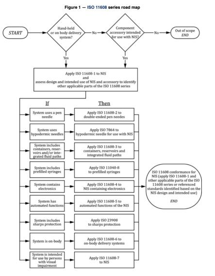
Figure 1: Road map of the ISO 11608 series that can be applied to different needle insertion systems.
