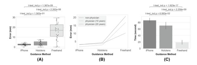
**Fig. 7** Results of experiment 2: comparison of needle placement performance. **a** Comparative box-and-whisker plot of the needle placement error for the AR smartphone, AR smartglasses, and CT-guided freehand navigation. Each dot represents a measurement of error for
