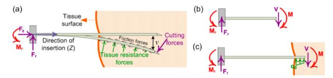
Figure 1: needle deflection in 2D. (a) Forces acting on the needle. (b) Shear force V and bending moment M at a cross-section just to the left of the tissue surface. (c) Shear force and bending moment at a cross-section just to the right of the tissue surface (inside the tissue)
