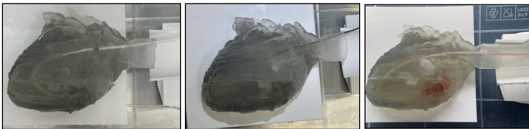
Figure 5. Wedge catheter, guide wire, and balloon catheter inserted in model (Left to Right)
