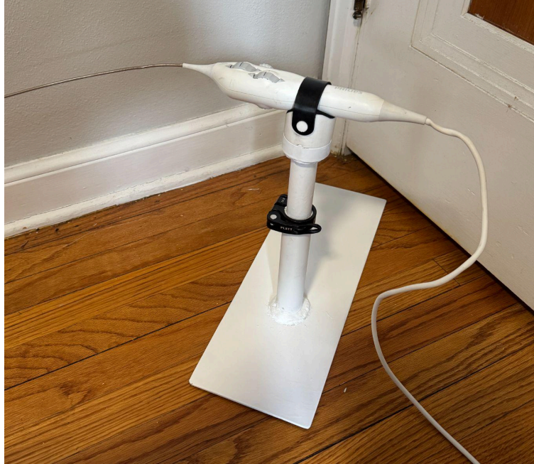
Fig. 11 Final fabricated prototype, consisting of top, middle, and base parts along with the pole clamp and 4D ICE catheter
