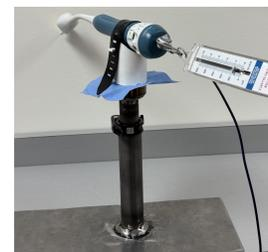
Fig. 8: Tensile force testing setup.
