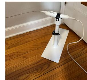
Fig. 5: Final prototype of device painted with top part angled and base and middle part off-centered
