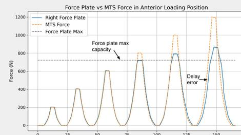
Figure 9. Force plate reading vs MTS reading with MTS loading in the anterior position with no shear load.
