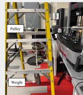
Figure 7. Pulley mechanism for shear loading during ramp and hold compression testing.
