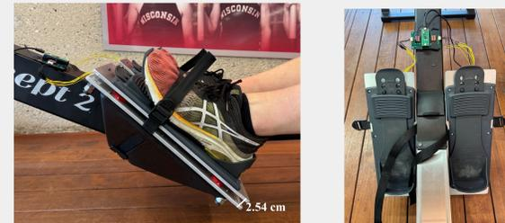
Figures 4 and 5. Side view and front view of force plates on ergometer.
