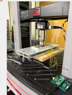
Figure 6. Normal compression loading test setup on MTS with plywood fixture.
