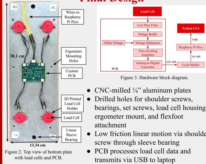
Figure 2. Top view of bottom plate with load cells and PCB.
