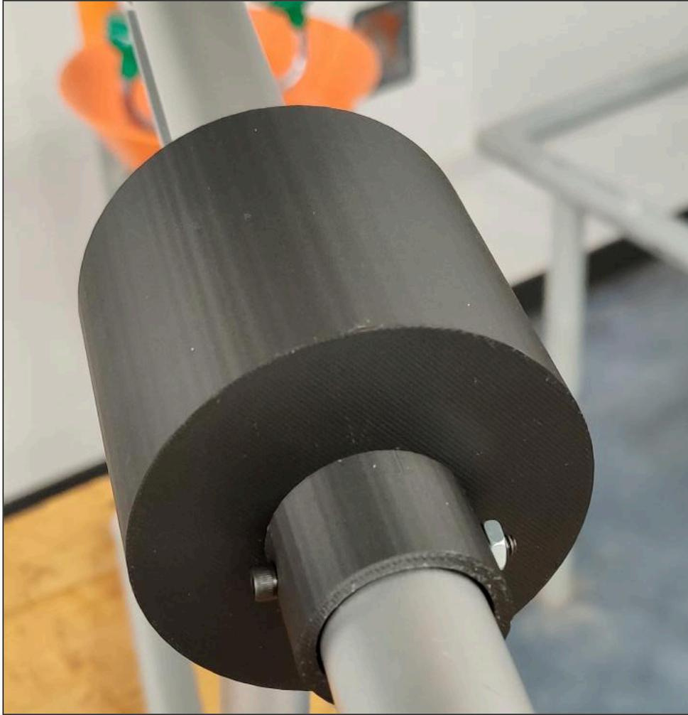
*Figure 9. Bolt mounting for the load cell holder.*
