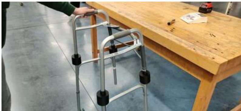
*Figure 10. Load cell holder assembly.*
