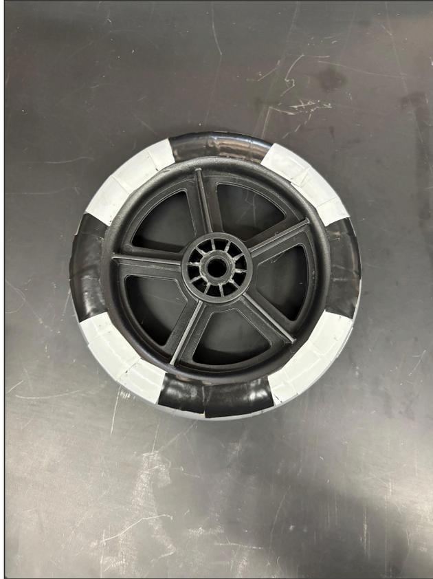
Figure 11. Inside of the walker wheel with 8 (4 of each) alternating colored taped strips.
