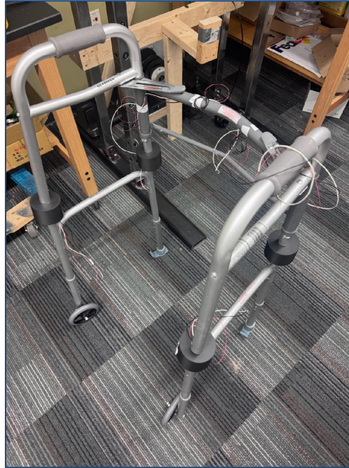
Figure 9. Current image of prototype featuring integration of load cell housing with walker
