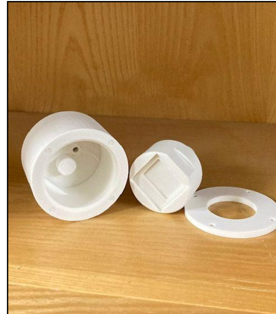
Figure 7. 3D printed loading cell housing prototype
