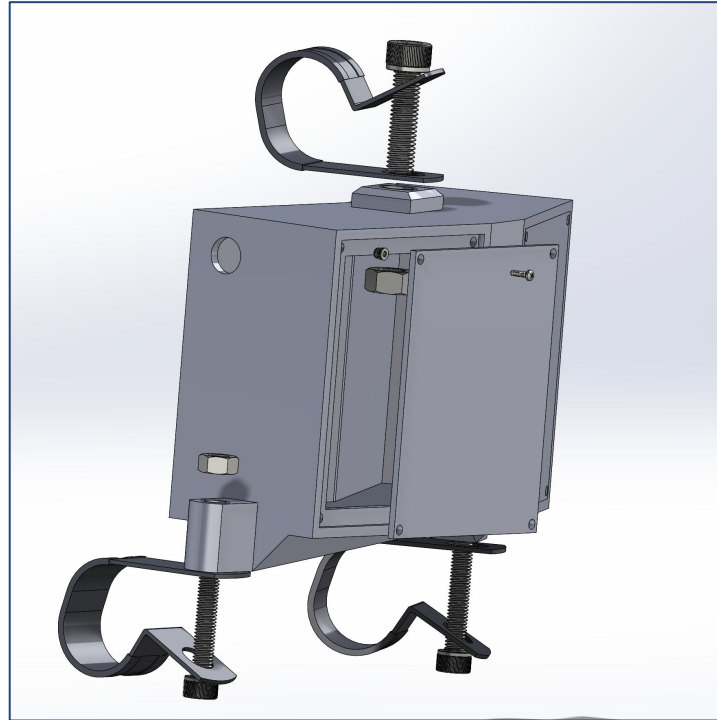
Figure 14. Electrical Housing with all Components
