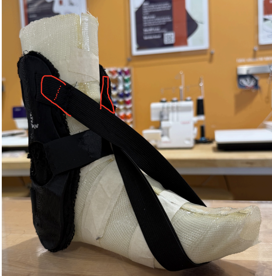
Figure 9: Dorsiflexion straps sewn to the brace
