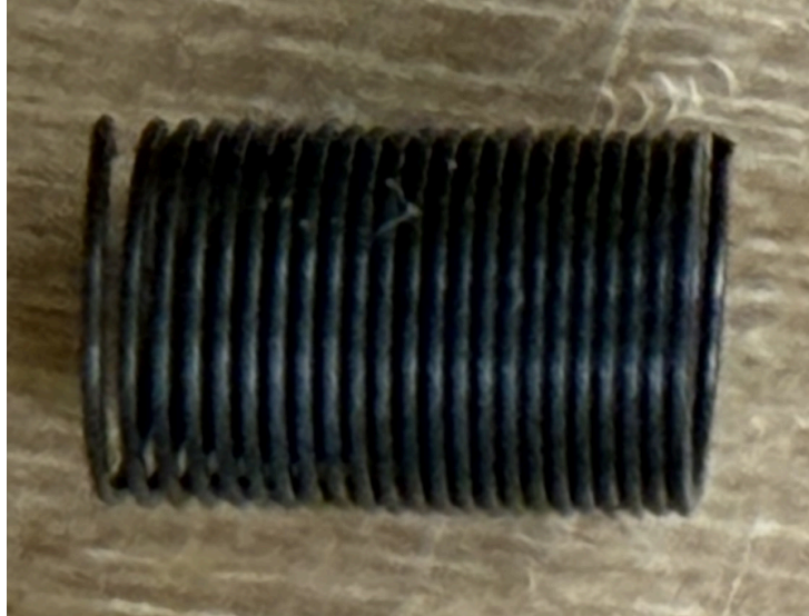
Figure 5. Nitinol spring prototype used to evaluate rollback behavior and increased surface interaction during eversion.
