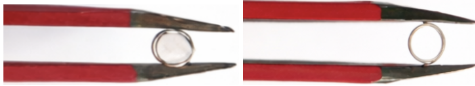
Figure 6. Comparison of cuff diameters in the compressed state (2.87 mm, left) and uncompressed state (4.19 mm, right).
