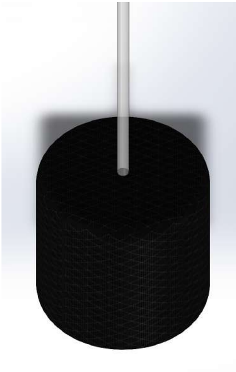
Figure 3. Degradable coating design after deployment. There is no longer a coating and the sponge has expanded to size.
