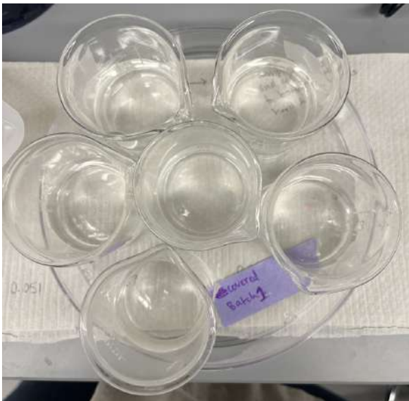
Figure 2. Covered gelatin samples dissolved after 10 minutes.
