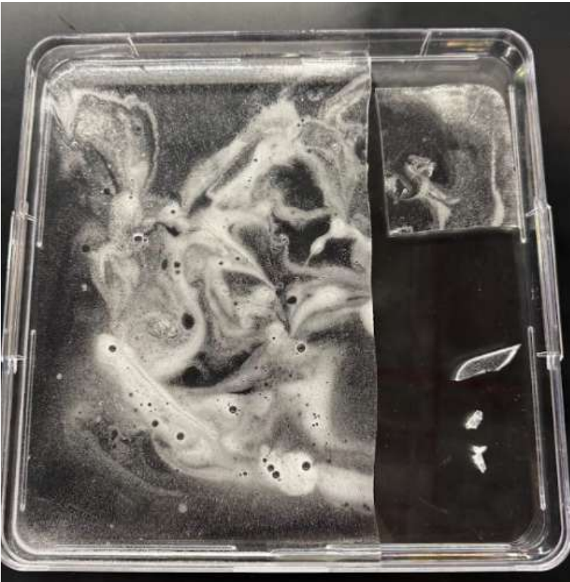
Figure 3. 25 cm by 25 cm gelatin sheet used to encapsulate sponge.
