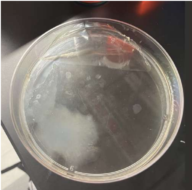
Figure 1. Film as I was taking it out of the dish. It was very strong and withstood me pulling it out with a tweezers. There are some spots where it got stuck, but I think that is where the last alginate did not evaporate. Additionally, it did not dry evenly so some spots were still gel.
