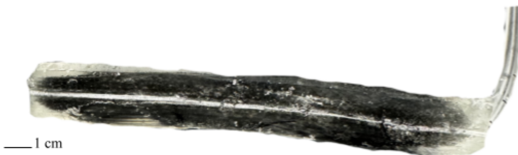
Figure 7: Final prototype of gelatin encapsulating polyurethane sponge.
