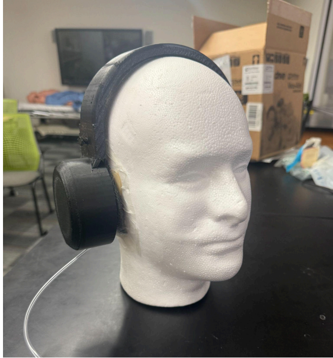
Figure 1. 3D printed EarVac device on foam head for testing
