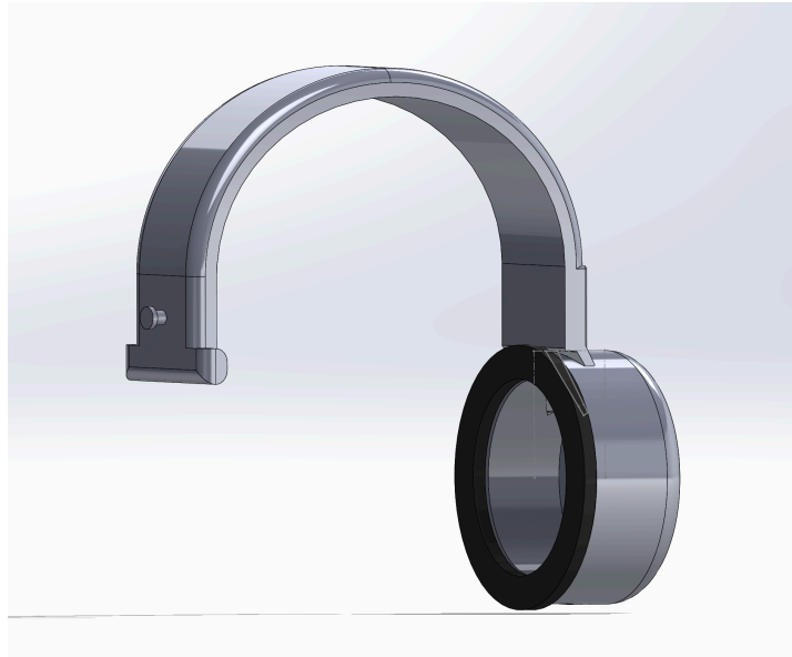
Figure 12. SolidWorks model of final design, interior of earmuff included
