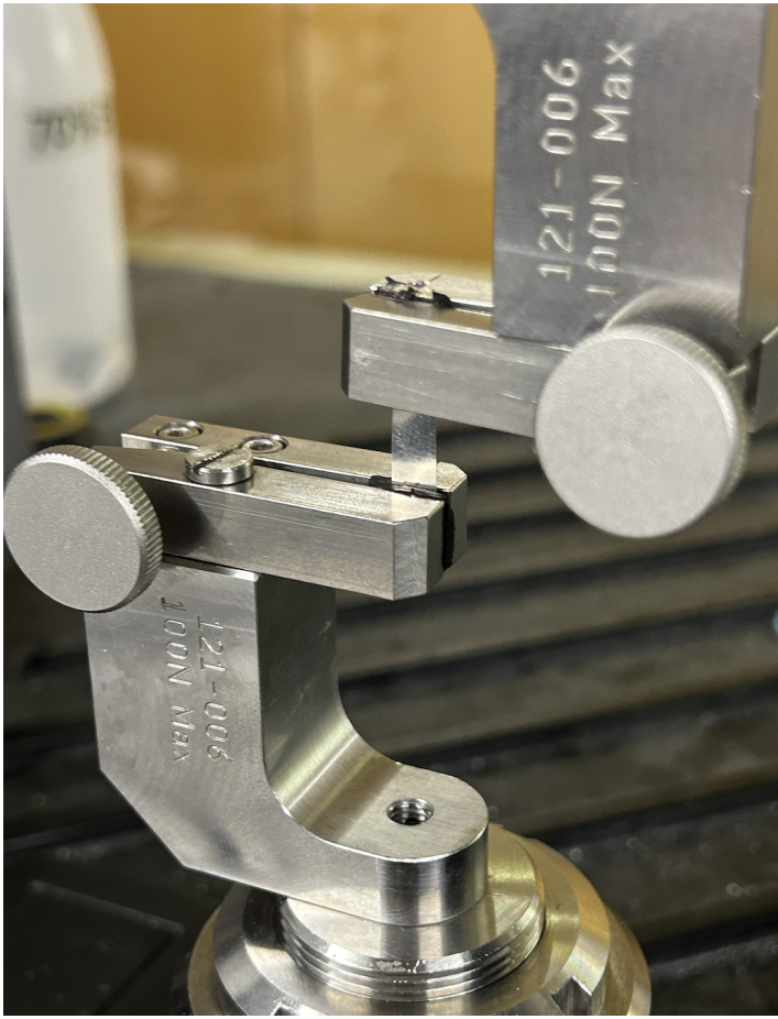
Fig. 2. Circumferential matrix sample loaded into the MTS machine.
