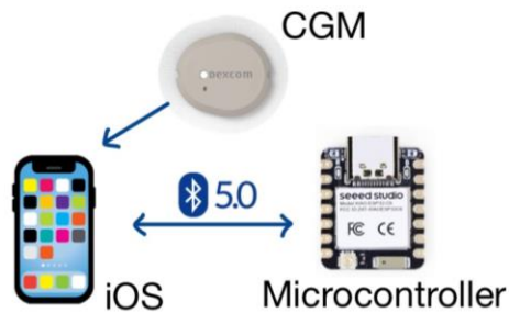
Figure 6: BLE 5.0 Only Connection
