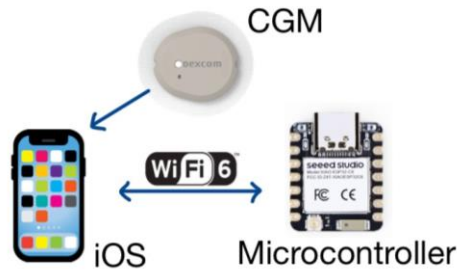
Figure 7: Wi-Fi 6 Only Connection
