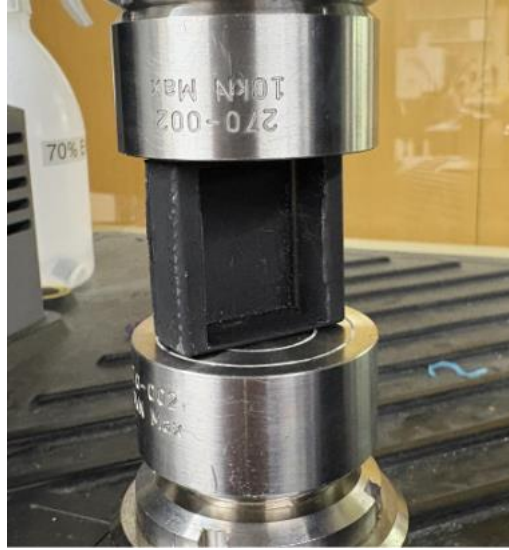
Figure [16]: MTS Testing Orientation of Device Watch Face with Resin Material
