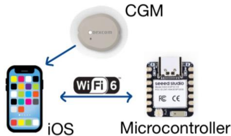
Figure 7: Wi-Fi 6 Only Connection
