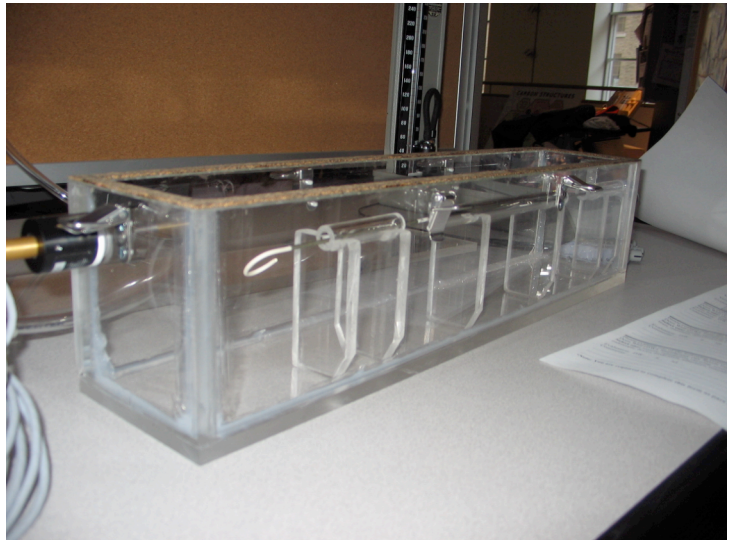
Figure 8: Close up of the container. This picture shows the tubular catheter mounts as well as the wall-mounted pressure sensor and cork gasket.
