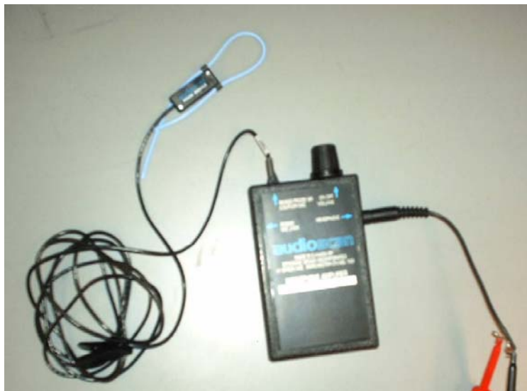
Fig 1. Audioscan Microphone pack. The microphone portion has a small loop that fits around the ear. The amplifier pack can be connected to the oscilloscope.
