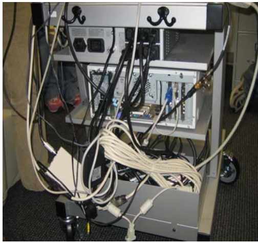
Figure IV: A view of the loose cords from the EEG components on the current cart.
