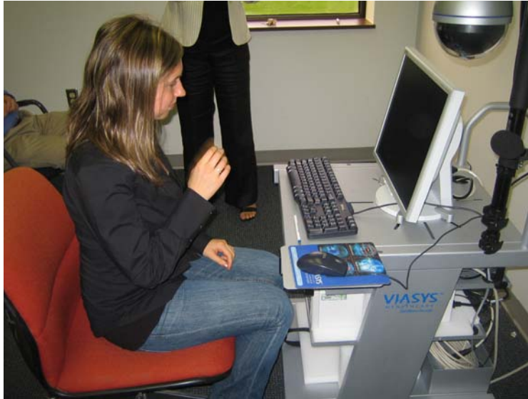
Figure XI: Here you can see the limited knee space when sitting at the current Viasys cart. With a sliding keyboard moved under the cart, there will more knee space to make working at the cart much more comfortable.
