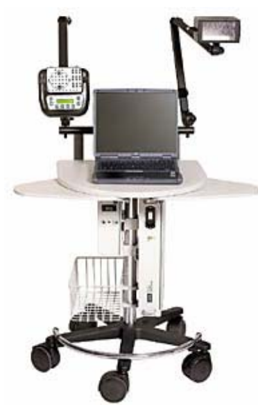
Figure VI: This cart from Grass-telefactor is very compact with a small footprint, but has minimal workspace and storage. The wings are also awkward and intrusive [4].
