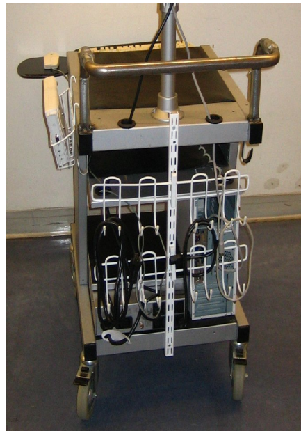
Figure XVIII: Here you can see the final design from the front and back. The front features rearranged components, sliding keyboard, and mounted monitor. The back features the adjustable push-bar, cable management, and additional storage.
