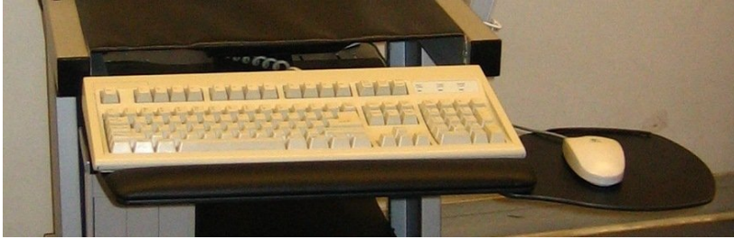
Figure XXI: The keyboard is now on a sliding keyboard tray with a swivel mouse pad. The keyboard tray allows for knee space when sitting and frees up surface space. The keyboard tray can also be accessed at a comfortable standing height.
