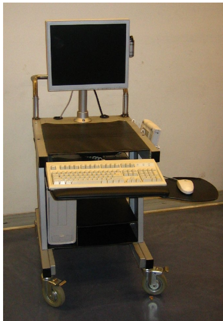
Figure XVIII: Here you can see the final design from the front and back. The front features rearranged components, sliding keyboard, and mounted monitor. The back features the adjustable push-bar, cable management, and additional storage.
