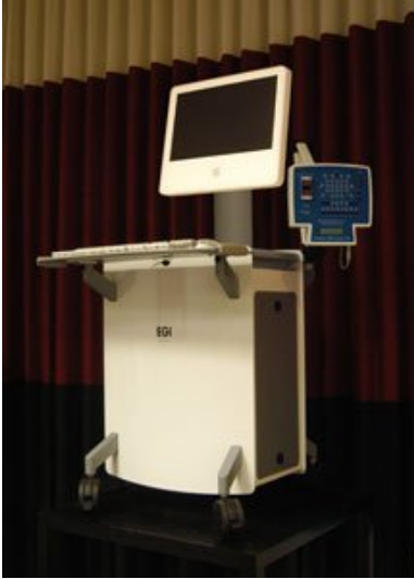
Figure VIII: This cart from EGI gives a neat appearance, but is somewhat bulky and has minimal workspace. [9]
