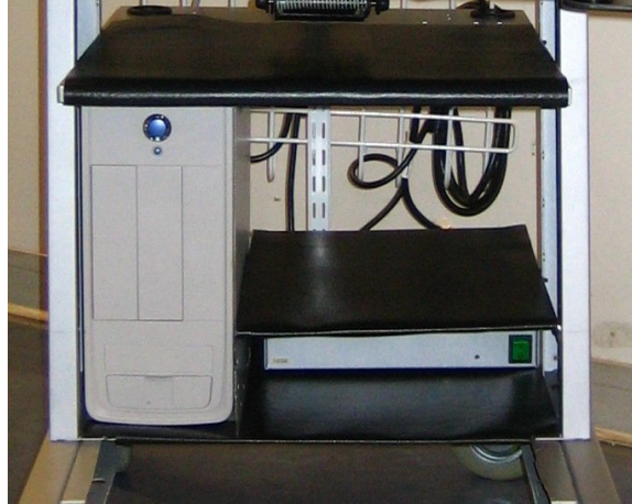
Figure XXII: Here you can see the components have been rearranged. The CPU now sits vertically and the power box is on the bottom shelf. This optimizes space.
