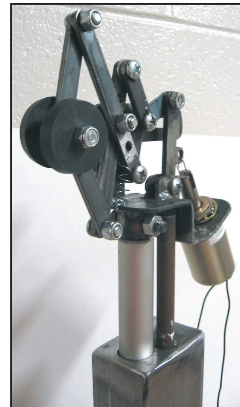
Figure 1. Prototype constructed in spring of 2006 including a linear actuator for height adjustment and a six-bar mechanism to press elevator buttons.
