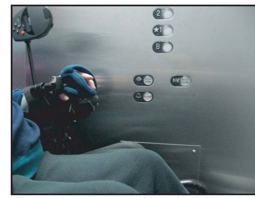
Figures 3 & 4. Stationary bar on base of user's wheelchair (left) and photo illustrating the typical position of the user's wheelchair while in the elevator cab, aligning the knee region of the chair with elevator buttons.
