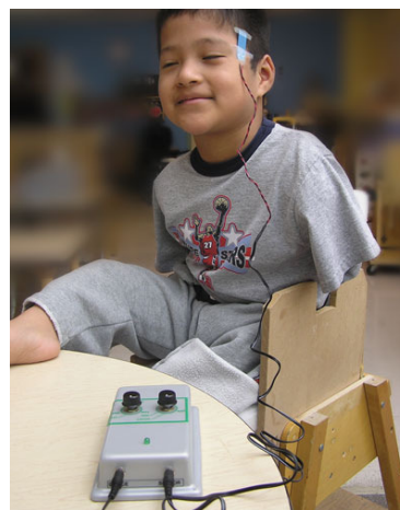
Figures 6 & 7. Examples of tongue switch (left) and eyebrow twitch switch (above) distributed by Enabling Devices
