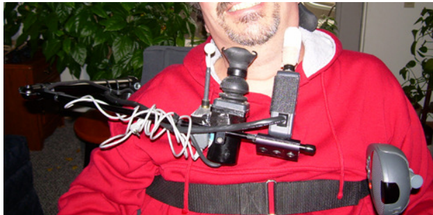
Figure 3. Graphic depicting detail of control bar on user's wheelchair, which currently includes a chin joystick for total control of chair movement, a tilt joystick to change the angle of the seat, and an unused lever previously connected to the user's telephone system.
