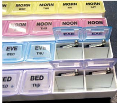
Figure 4. Painted copper plates prevent pills from interfering with switch circuitry.
