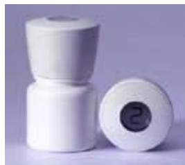
Figure 1. Medication Event Monitoring System records when a single vial is accessed by a patient.
