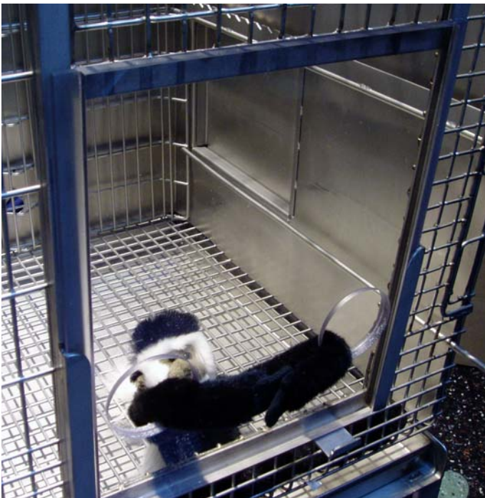
Figure 7: Adapter panel. Shown with monkey model reaching through holes.
