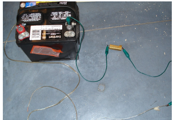
Figure 3: Battery and Power Resistor in Series
