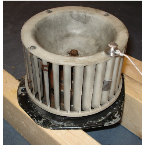
Figure 4: Fan Motor Bolt, washer, and string attached through outer rim of fan
