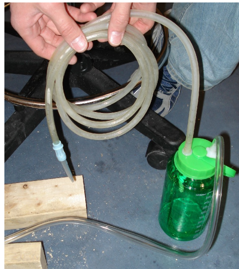
Figure 6: Collection Chamber, Tubing, and Autoclavable Tip
