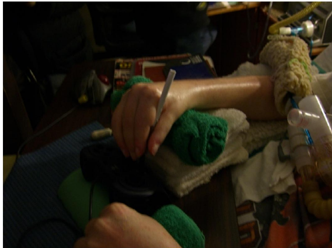
Figure 9. Game controller with adapted and jointed joystick. Client is seen using the device for the first time.
