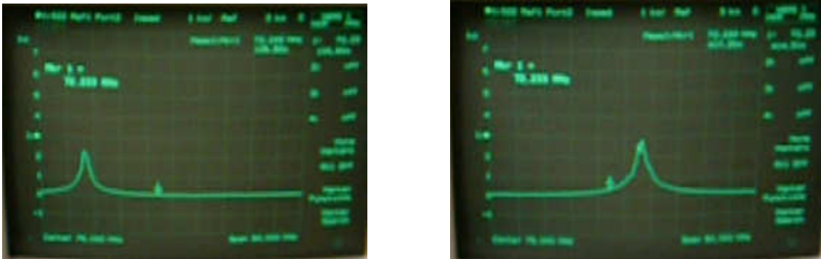
Figure 28. Resonant frequency peaks measured on oscilloscope.
