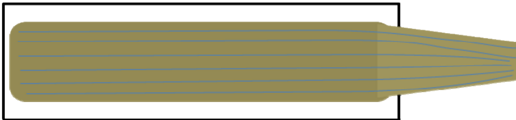
Figure 8: Focusing the Magnetic Field by Narrowing Ferromagnetic Core
