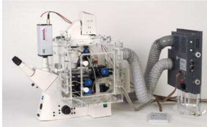
Figure 3. EMBL Live Cell Observation Chamber by CellBiology Trading (Kern, 2007).
