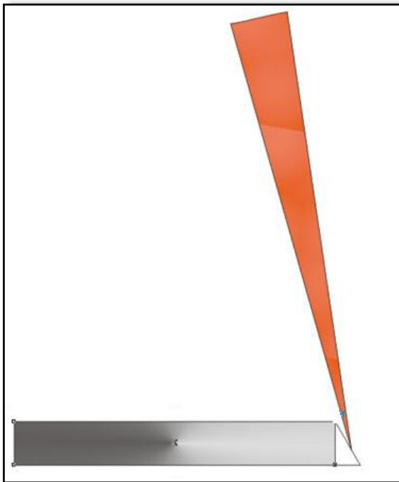
Figure 1: Prism (field of view 6.385 degrees); field of view is to scale. The rectangle represents the exterior of the needle and the triangular portion is the total field of view.
