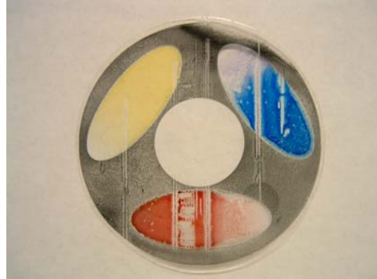
Figure 9: Picture of the final product. It has lines without color due to scraping by the printer.
