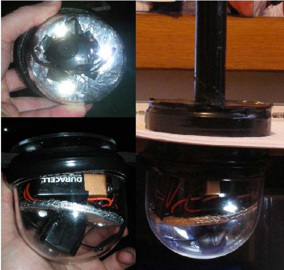
Figure 10: Photos of the finished prototype; the dome camera with illuminated LEDs (top left); the 9V power source held down to the base of the camera (bottom left) and the final magnetic couple system held between sheets of notebook paper (right).
