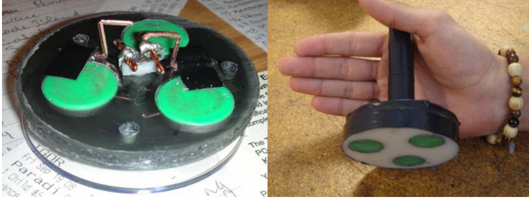
Figure 7: Magnetically-induced Pressure Switch System (left) coupled with magnetic scope (right).
