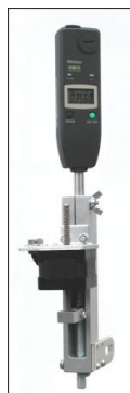
Figure 4: A solution valve opener allows controlled flow of a chemical (Audie Technology, 2008).
