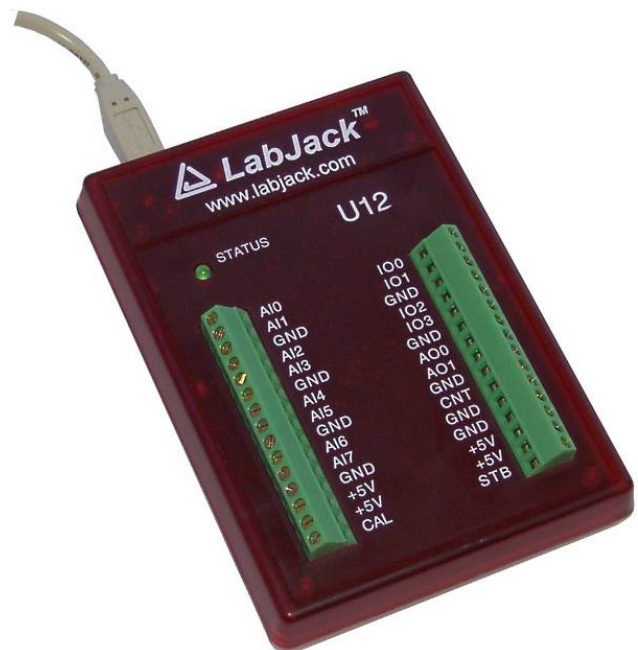
Figure 3: LabJack U12 interface [1]. Allows signals sent from program to activate each valve. Low voltage digital I/O signals from device must first be boosted to meet valve requirements.
