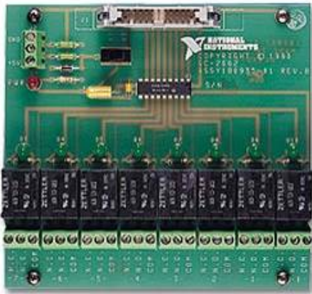
Figure 4: NI SC-2062 Power Relay Board [2]. Boosts the low voltage output from the LabJack U12 device to the 12 VDC necessary to drive each valve.
