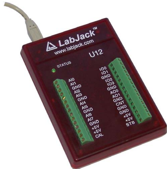
Figure 8: LabJack U12 interface. Sends low voltage signals to turn on/off each valve. Low voltage digital I/O signals from device must first be boosted to meet valve requirements [2].
