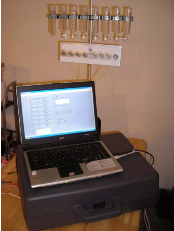
Figure 11: Flow rate test set up. Set up is similar to client's working conditions
