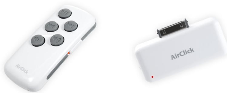
Figure 2: Air Click by Griffin Technologies [1] with five button layout for navigation, play/pause, and volume control
