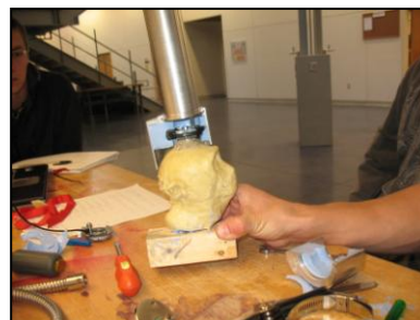
Figure A-2: Clamping half of the silicone rubber interior and aluminum base to the base of the microdrive unit and attaching cylindrical top
