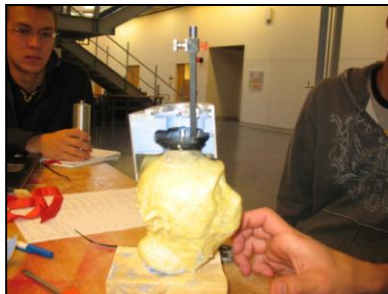
Figure A-1: Clamping half of the silicone rubber interior and aluminum base to the base of the microdrive unit
