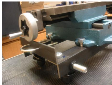
Figure 8: ¼ view of the final design from the side depicting the crank mechanism used to move the platform and the U-bolt required to facilitate rotation
