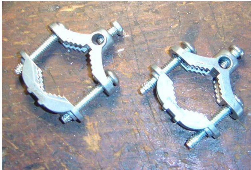
Figure 8: Electrical ground clamps used in design. Part with one screw is referred to as the top.
